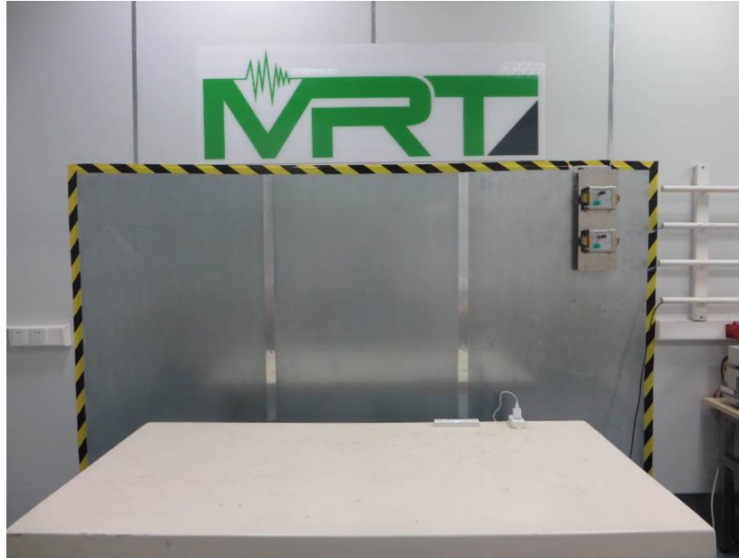
Set-up for Conducted Emission
