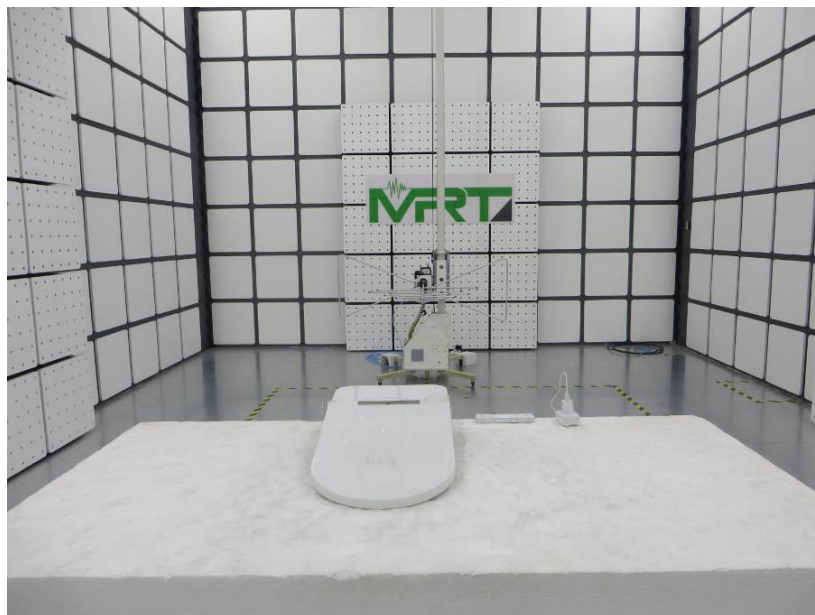
Set-up for Radiated Emission
