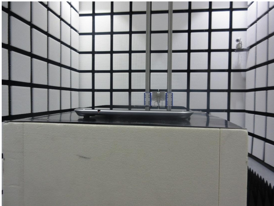
Radiated Emission Test Above 1GHz
