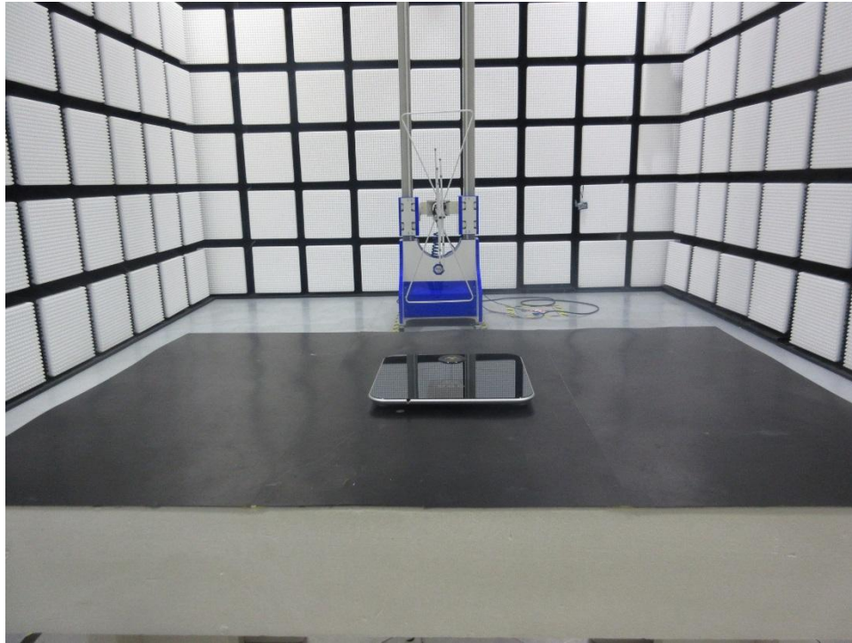
Radiated Emission Test Below 1GHz
