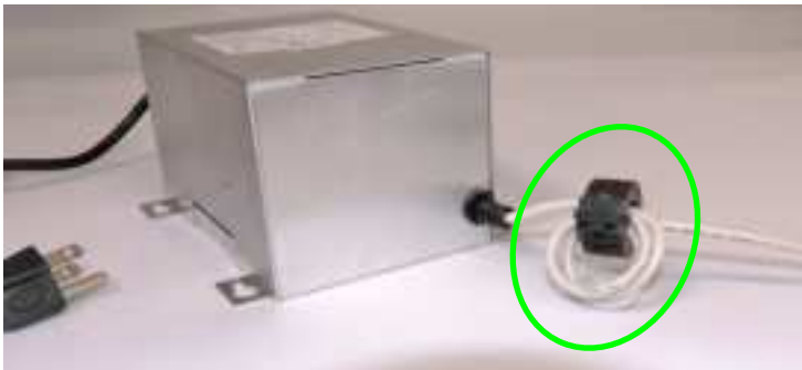
Figure 5: Optional Ferrite Core Placement, Near PSU Adapter
