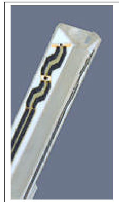
Inside view of ET3DV6 E-field Probe
