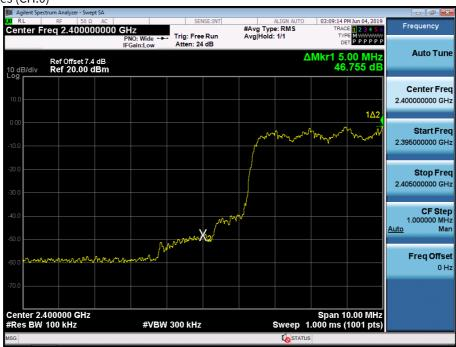
Test Plots with hopping ( $\pi/4DQPSK$ )
