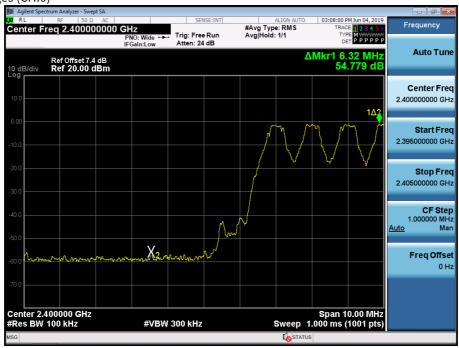
Test Plots with hopping (GFSK)
