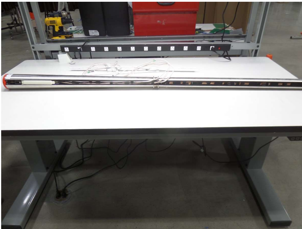
Figure 1: NS40 antenna with plastic strips removed
