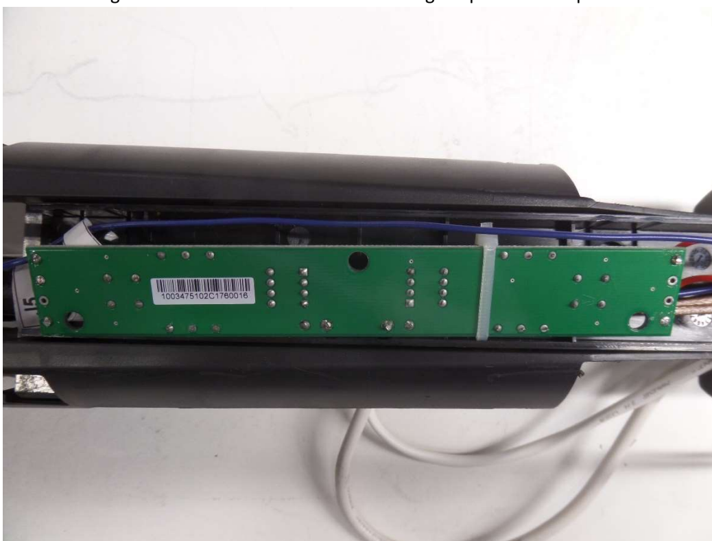
Figure 12: NS40 antenna A1200 matching coupler board bottom side
