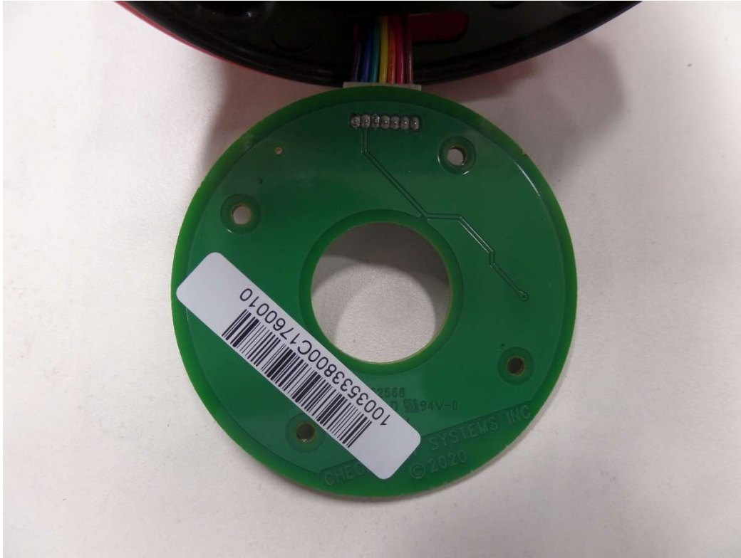
Figure 19: NS40 antenna pedestal A1198 LED board bottom side
