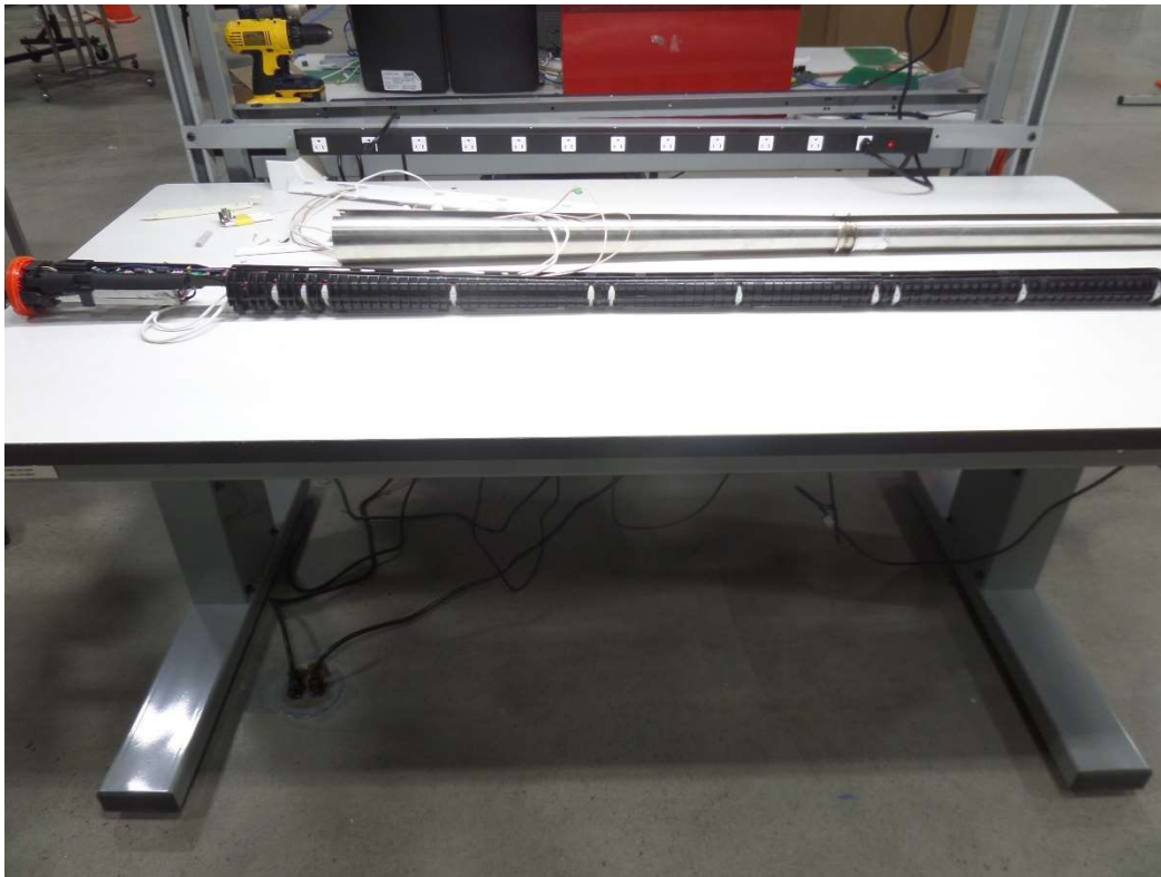
Figure 5: NS40 antenna without the metal housing
