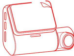
Press the dash cam against the attached electrostatic sticker to secure the dash cam.
