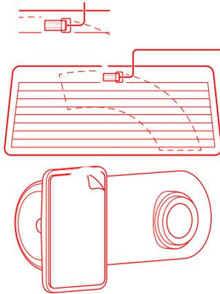
Press the rear camera against the rear windshield to secure the rear camera.
