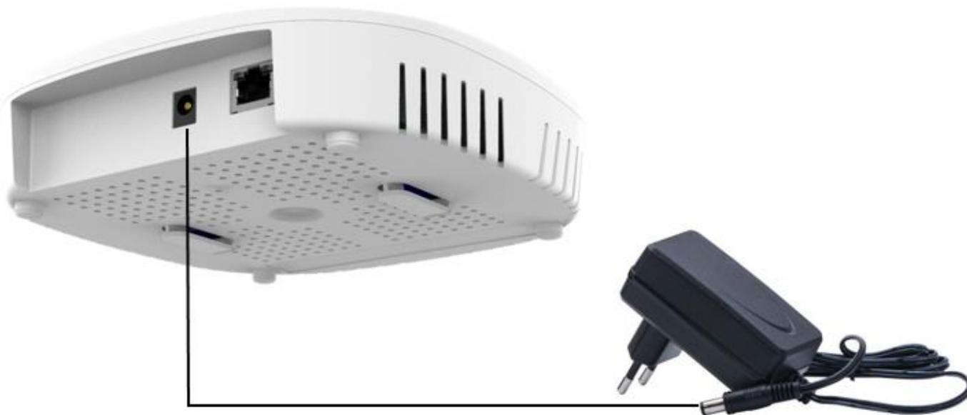
*Figure 6: Power up Indoor device using DC adaptor*
