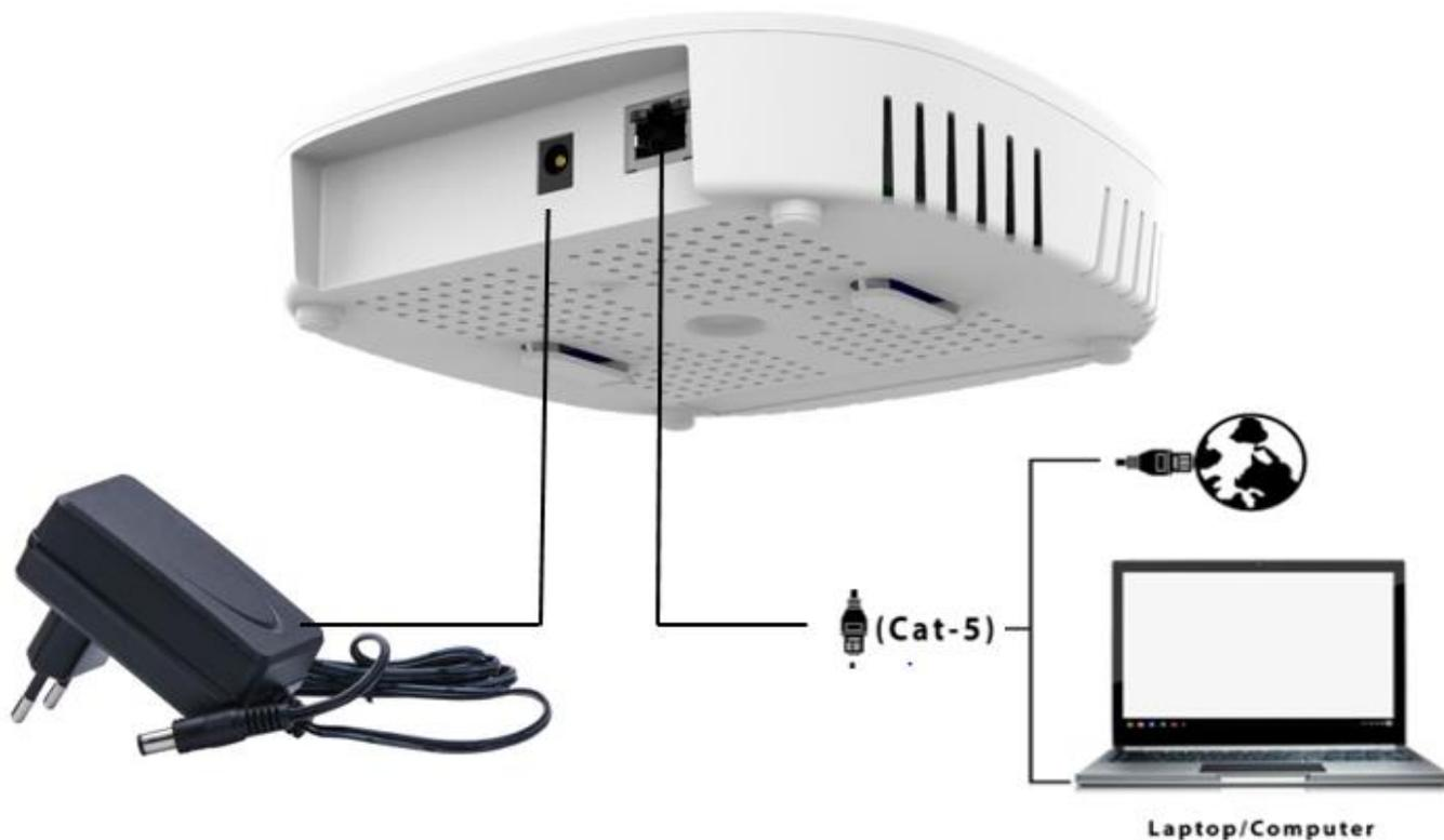
Figure 7: Connect Indoor Device to the network
