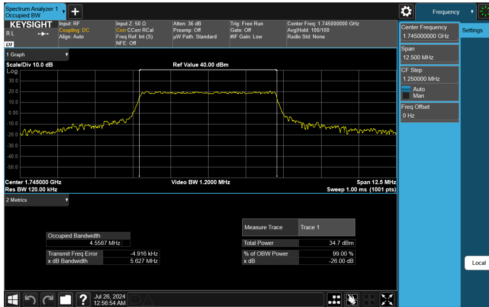
Plot 7-9. Occupied Bandwidth Plot (LTE Band 66/4 - 5MHz QPSK - Full RB)
