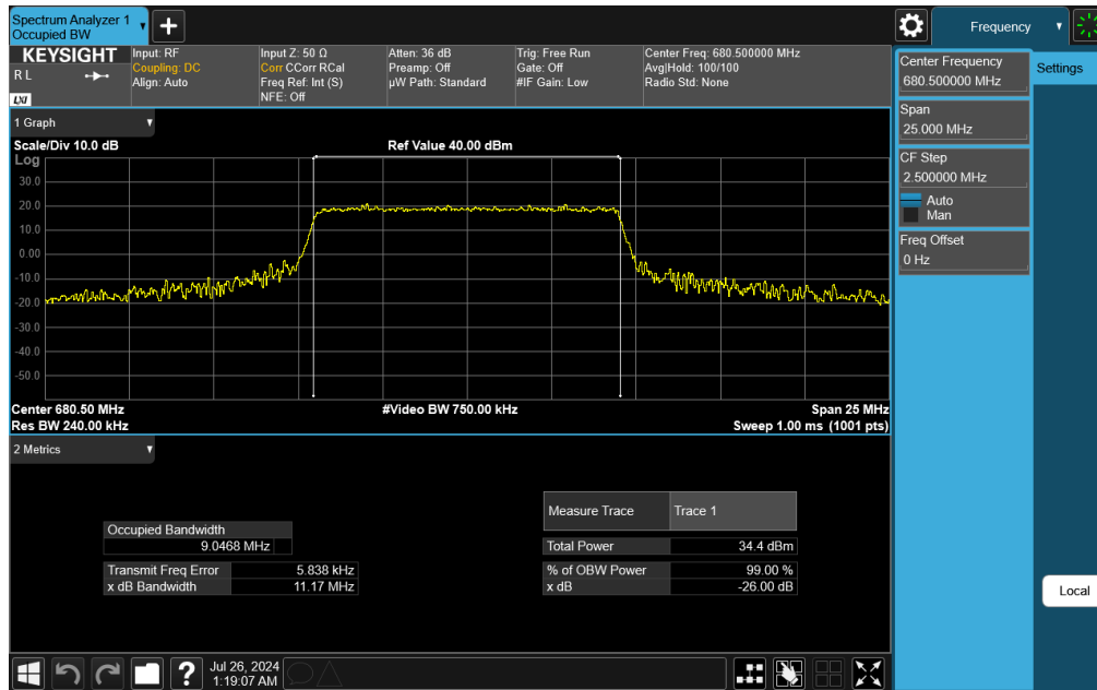
Plot 7-29. Occupied Bandwidth Plot (LTE Band 71 - 10MHz QPSK - Full RB)
