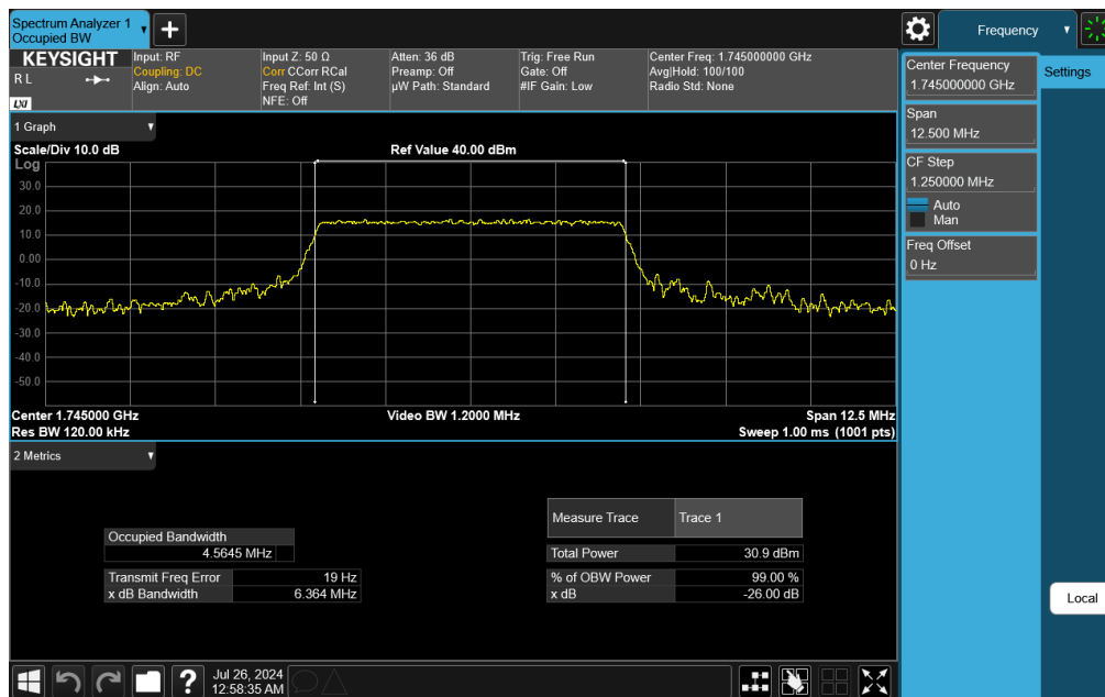
Plot 7-12. Occupied Bandwidth Plot (LTE Band 66/4 - 5MHz 256-QAM - Full RB)
