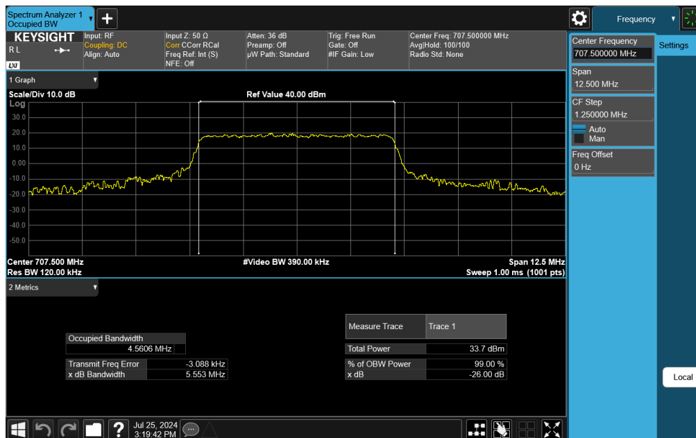
Plot 7-50. Occupied Bandwidth Plot (LTE Band 12/17 - 5MHz 16-QAM - Full RB)
