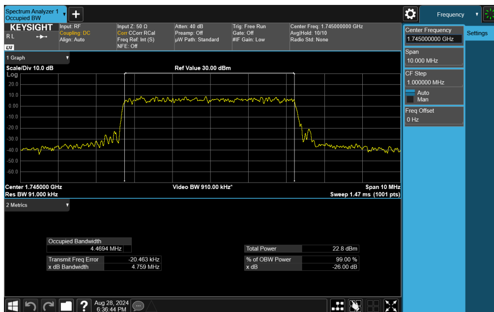
Plot 7-66. Occupied Bandwidth Plot (NR Band n66 - 5MHz CP-OFDM QPSK - Full RB)
