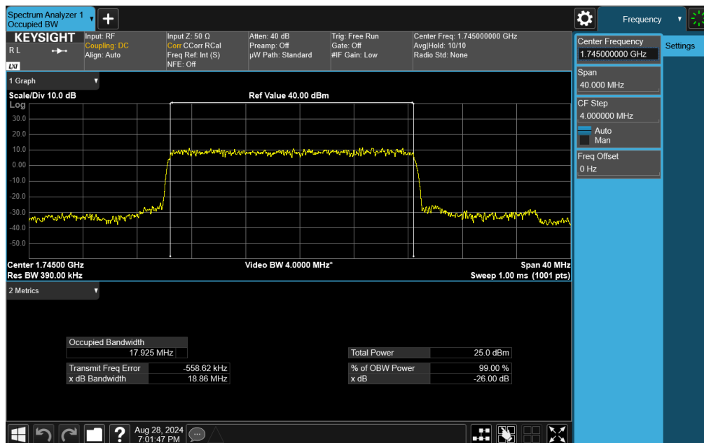
Plot 7-80. Occupied Bandwidth Plot (NR Band n66 - 20MHz DFT-s-OFDM \pi/2 BPSK - Full RB)
