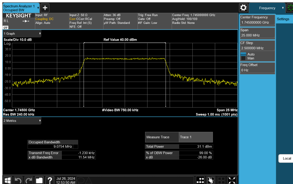
Plot 7-16. Occupied Bandwidth Plot (LTE Band 66/4 - 10MHz 256-QAM - Full RB)
