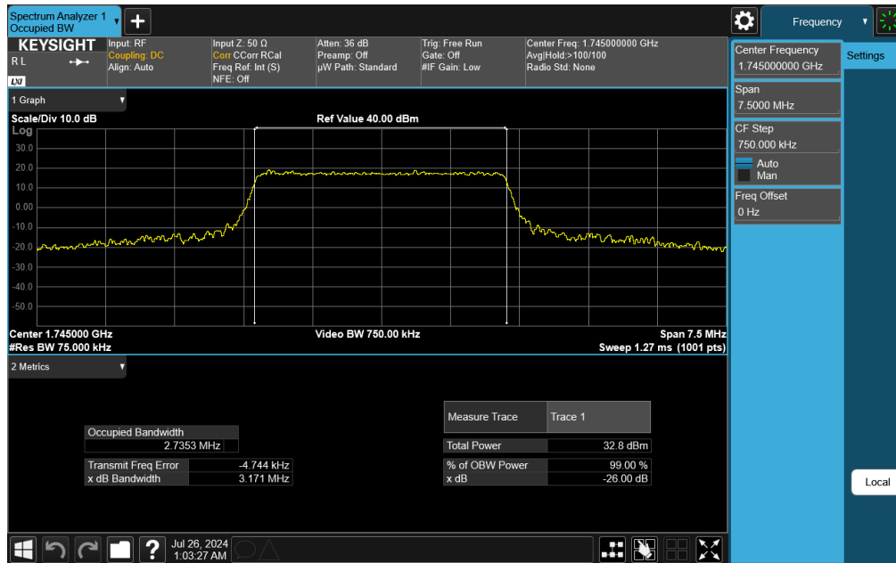
Plot 7-7. Occupied Bandwidth Plot (LTE Band 66/4 - 3MHz 64-QAM - Full RB)
