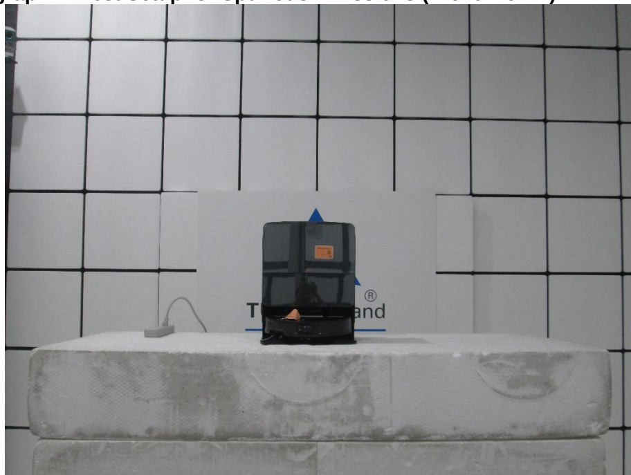
Photograph 2: Test Setup for Spurious Emissions (Front View 2)
