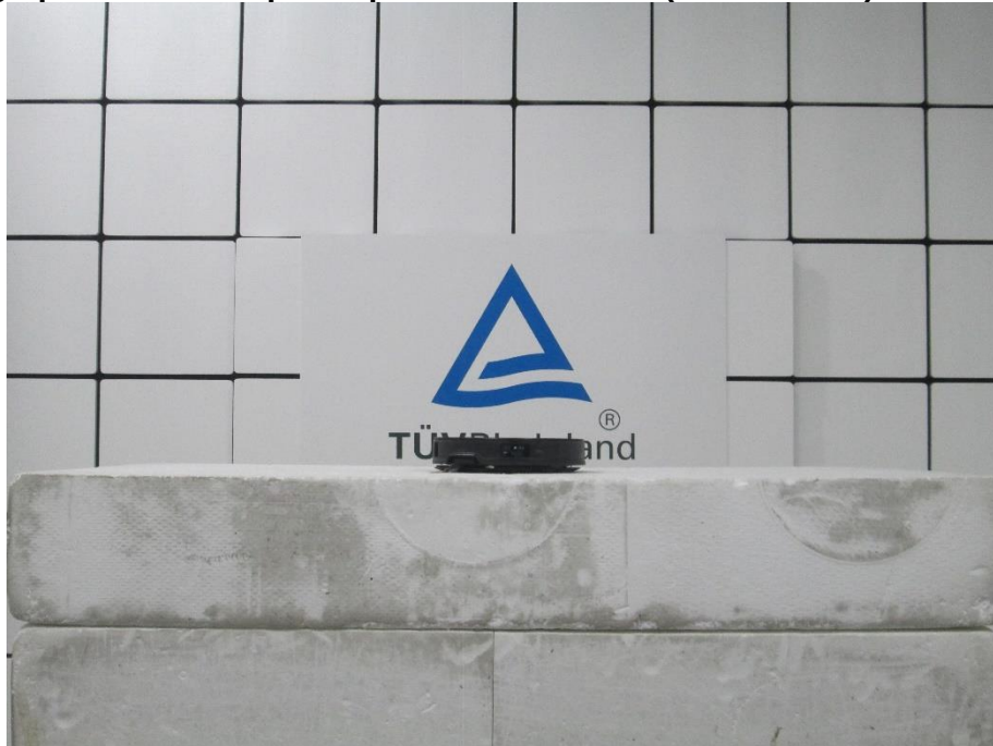
Photograph 7: Test Setup for Spurious Emissions (Front View 3)
