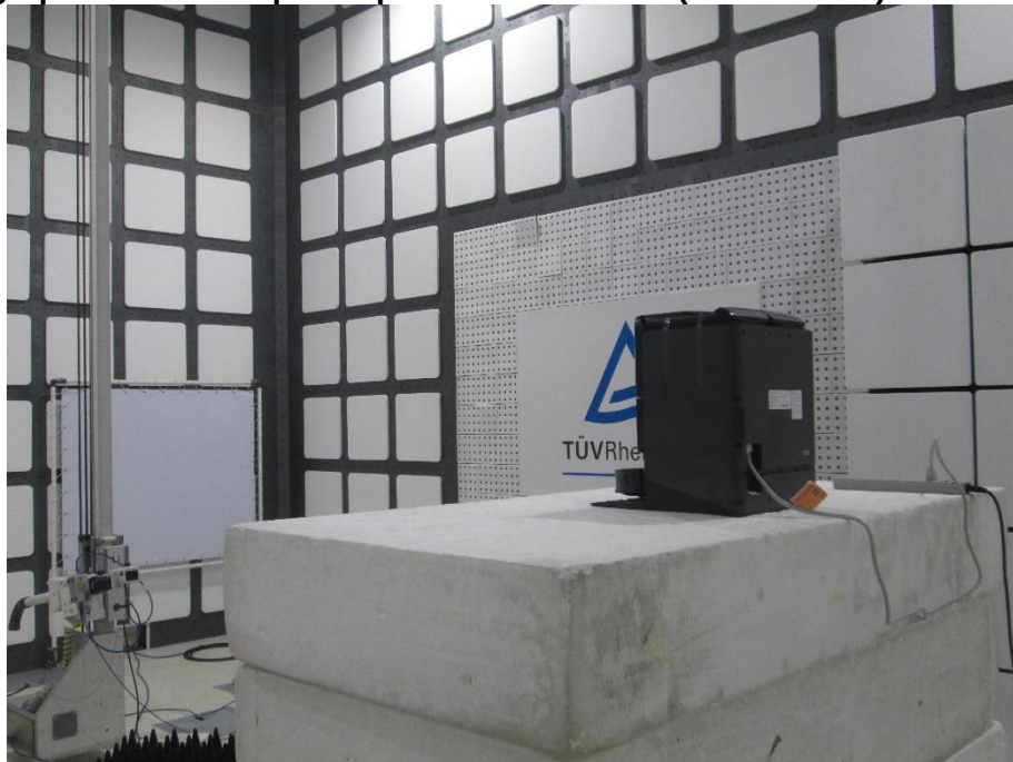
Photograph 6: Test Setup for Spurious Emissions (Back View 4)
