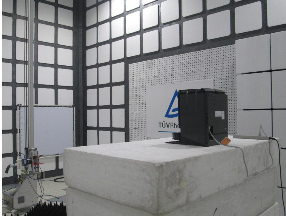
Photograph 6: Test Setup for Spurious Emissions (Back View 4)
