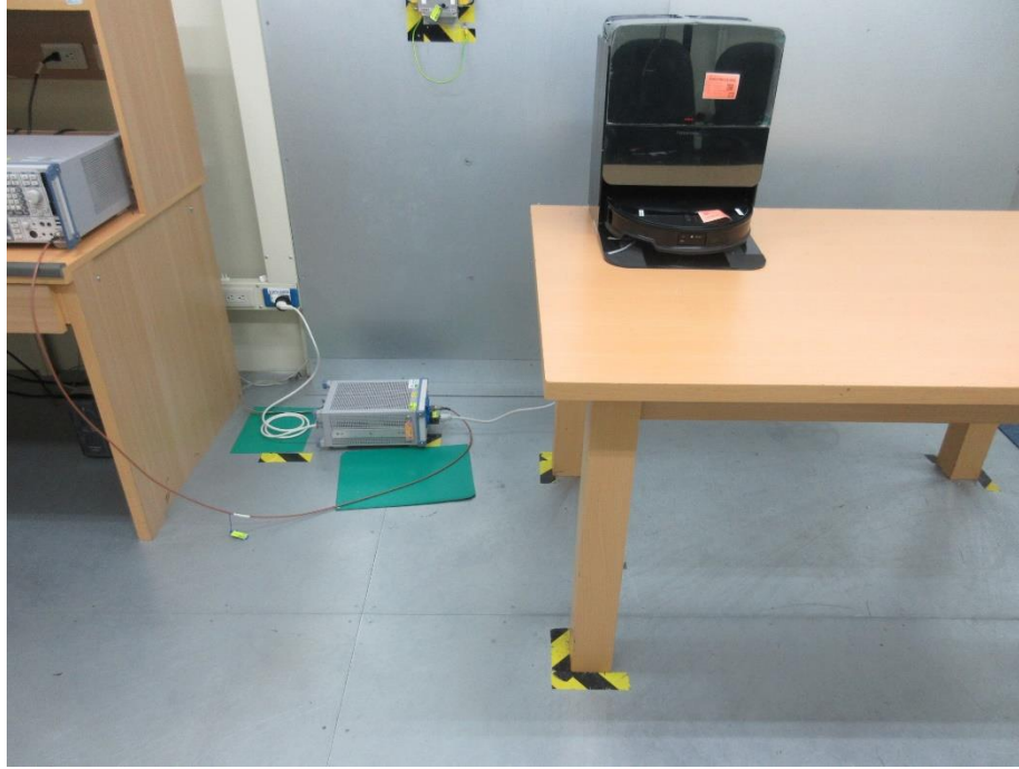
Photograph 9: Test Setup for Mains Conducted Emissions (Back View)
