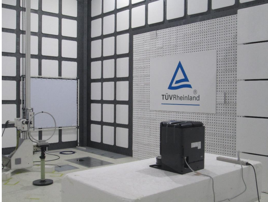
Photograph 3: Test Setup for Spurious Emissions (Back View 1)
