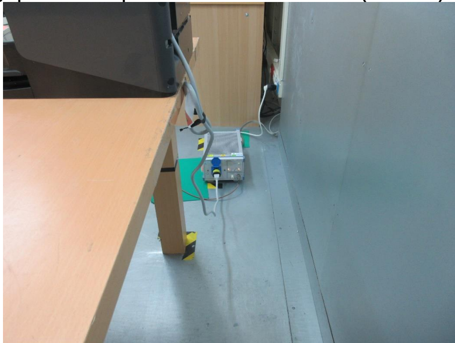
Photograph 9: Test Setup for Mains Conducted Emissions (Back View)
