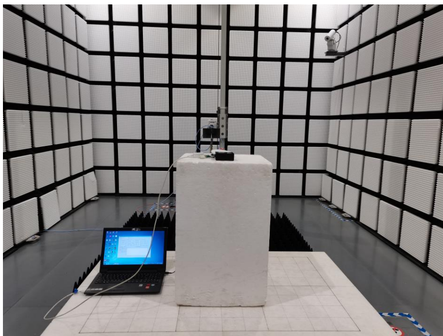
Fig. 3 Radiated emission setup photo(Above 1GHz)
