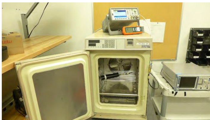
Figure D-1 - Test Setup for Frequency Stability
