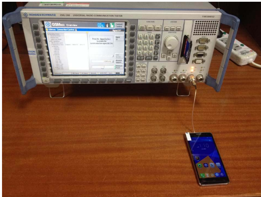
Photograph –2G&3G Conducted Test Setup
