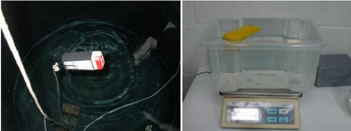
Figure 5 - Buoyancy test (FF right / SOLO left)
