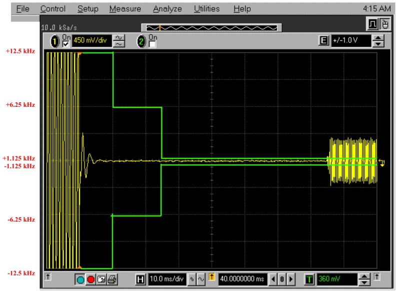
ANNEX 1 - PLOTS OF TRANSIENT FREQUENCY BEHAVIOR MEASUREMENTS PLOT # 28
