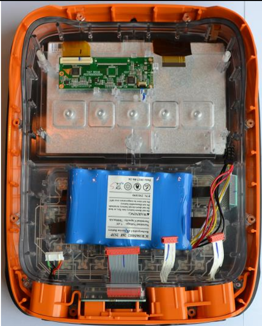
Internal Battery and LCD Module
