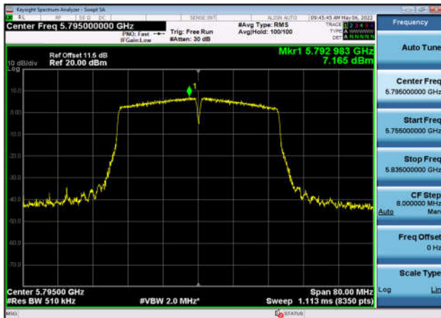
U-NII-3 Power spectral density-802.11 a(20MHz),5785MHz,Ant3
