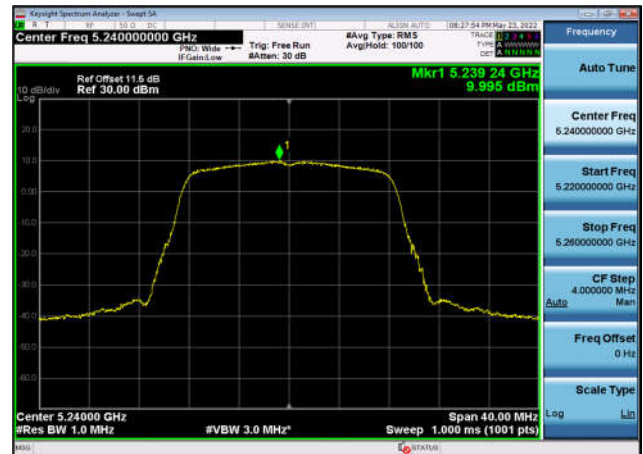
U-NII-1 Power spectral density-802.11 ac(20MHz),5220MHz,Ant3
