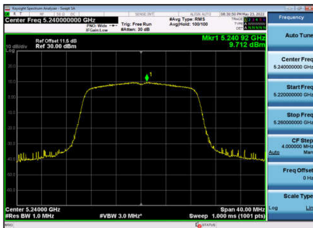
U-NII-1 Power spectral density-802.11 n(20MHz),5240MHz,Ant1
