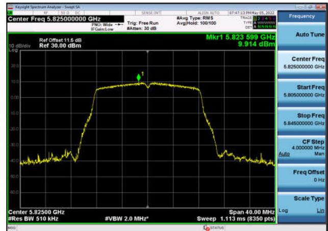
U-NII-3 Power spectral density-802.11 ac(20MHz),5785MHz,Ant2
