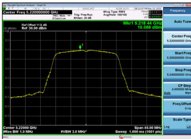
U-NII-1 Power spectral density-802.11 a(20MHz),5220MHz,Ant2
