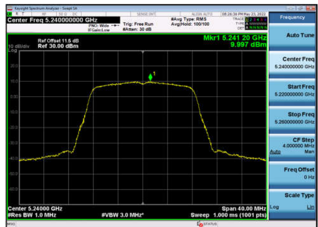
U-NII-1 Power spectral density-802.11 a(20MHz),5240MHz,Ant2
