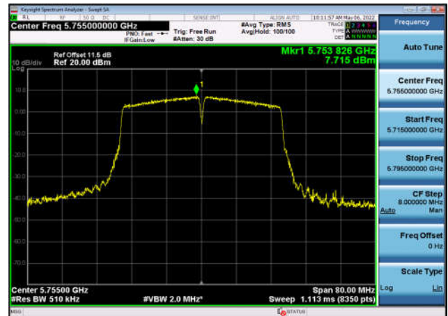
U-NII-3 Power spectral density-802.11 ax(80MHz),5775MHz,Ant0
