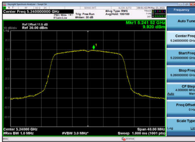
U-NII-1 Power spectral density-802.11 ac(40MHz),5230MHz,Ant1
