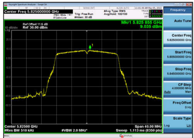
U-NII-3 Power spectral density-802.11 ac(20MHz),5785MHz,Ant0
