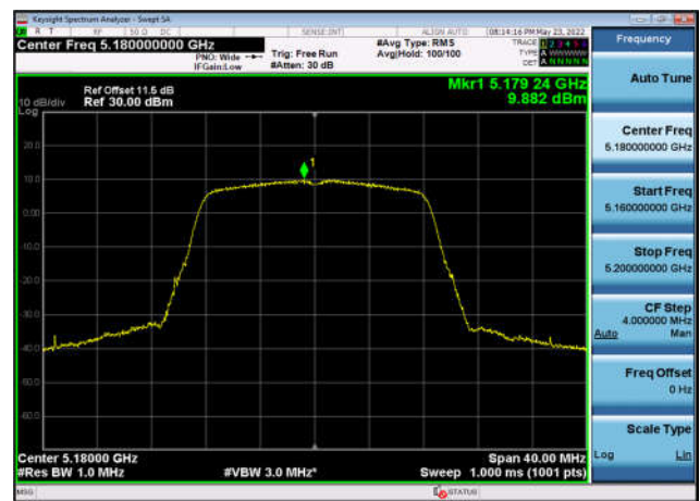
U-NII-1 Power spectral density-802.11 a(20MHz),5180MHz,Ant0
