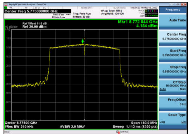
U-NII-3 Power spectral density-802.11 n(20MHz),5785MHz,Ant1
