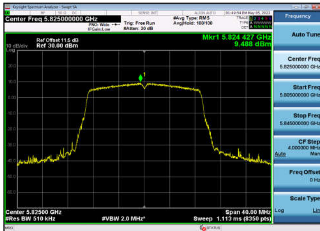
U-NII-3 Power spectral density-802.11 ac(40MHz),5795MHz,Ant0
