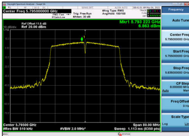
U-NII-3 Power spectral density-802.11 ax(20MHz),5745MHz,Ant2
