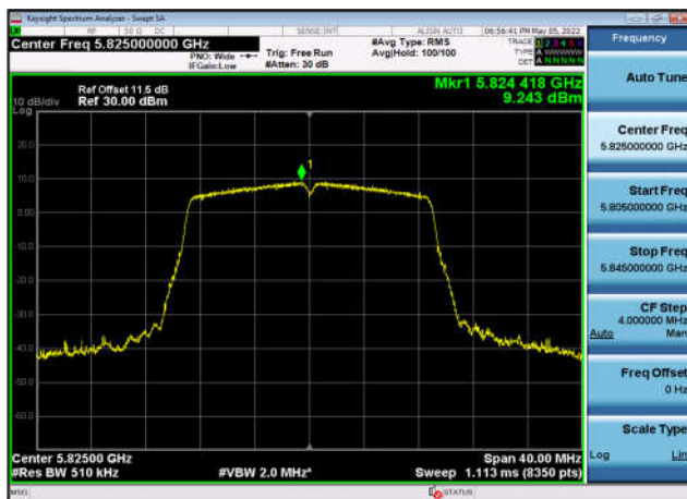
U-NII-3 Power spectral density-802.11 ac(20MHz),5825MHz,Ant2
