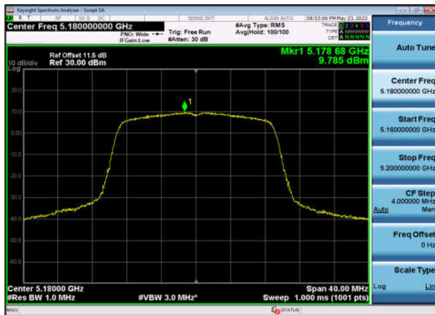
U-NII-1 Power spectral density-802.11 ac(20MHz),5240MHz,Ant0
