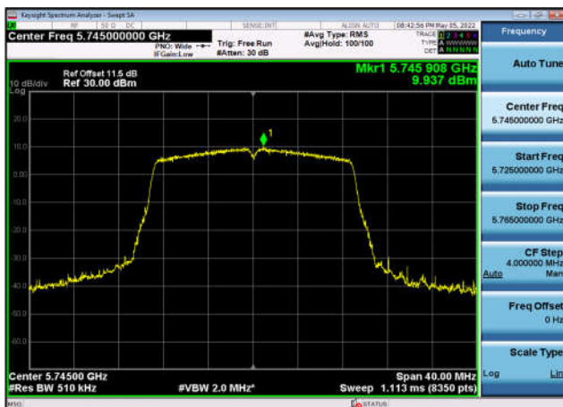
U-NII-3 Power spectral density-802.11 ac(20MHz),5745MHz,Ant3
