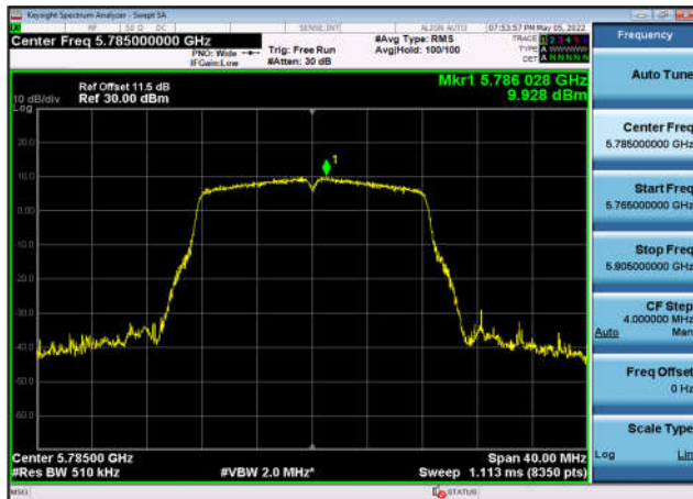
U-NII-3 Power spectral density-802.11 ac(20MHz),5745MHz,Ant2
