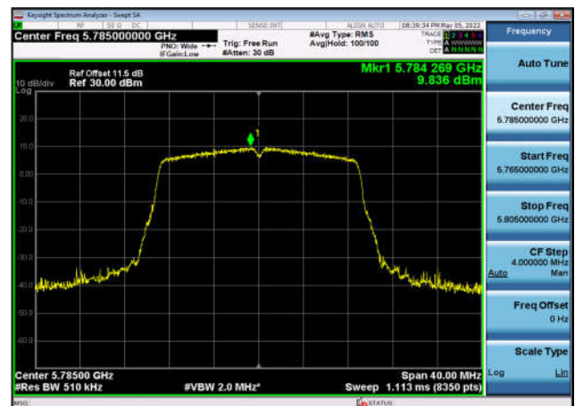
U-NII-3 Power spectral density-802.11 ac(20MHz),5785MHz,Ant3
