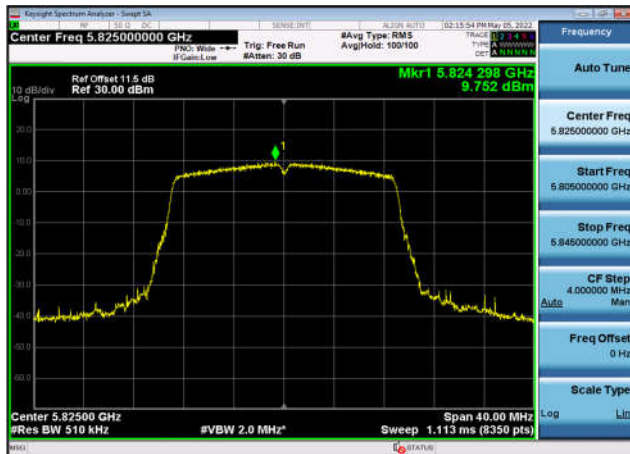
U-NII-3 Power spectral density-802.11 ax(40MHz),5795MHz,Ant0
