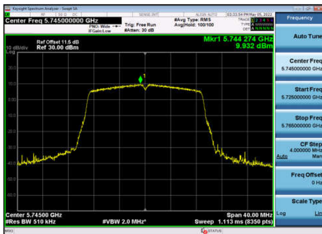
U-NII-3 Power spectral density-802.11 n(20MHz),5745MHz,Ant1
