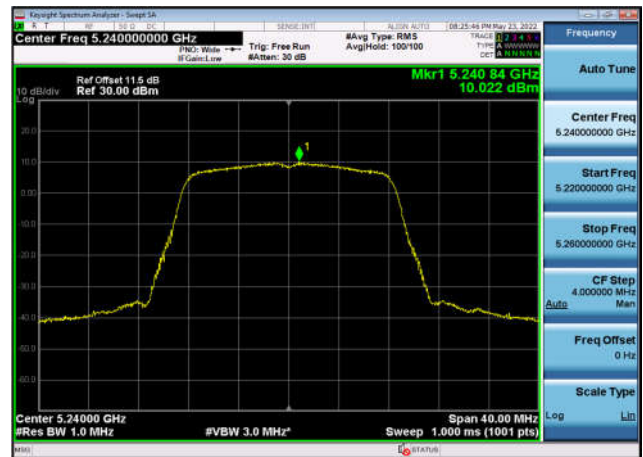
U-NII-1 Power spectral density-802.11 ac(20MHz),5220MHz,Ant1
