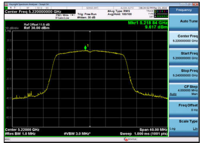
U-NII-1 Power spectral density-802.11 n(40MHz),5190MHz,Ant0
