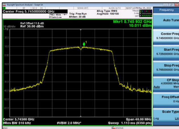
U-NII-3 Power spectral density-802.11 ax(20MHz),5745MHz,Ant3
