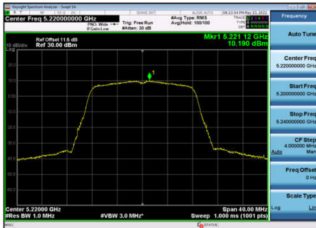
U-NII-1 Power spectral density-802.11 ac(20MHz),5180MHz,Ant3
