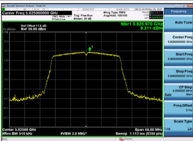
U-NII-3 Power spectral density-802.11 n(20MHz),5825MHz,Ant3
