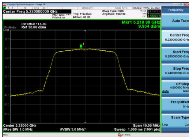
U-NII-1 Power spectral density-802.11 ac(20MHz),5180MHz,Ant1
