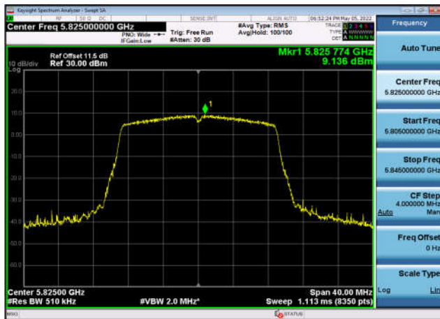
U-NII-3 Power spectral density-802.11 ac(40MHz),5795MHz,Ant1
