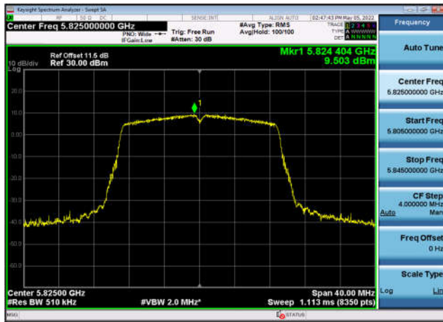
U-NII-3 Power spectral density-802.11 ax(40MHz),5795MHz,Ant3
