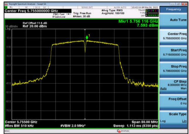
U-NII-3 Power spectral density-802.11 ax(80MHz),5775MHz,Ant3
