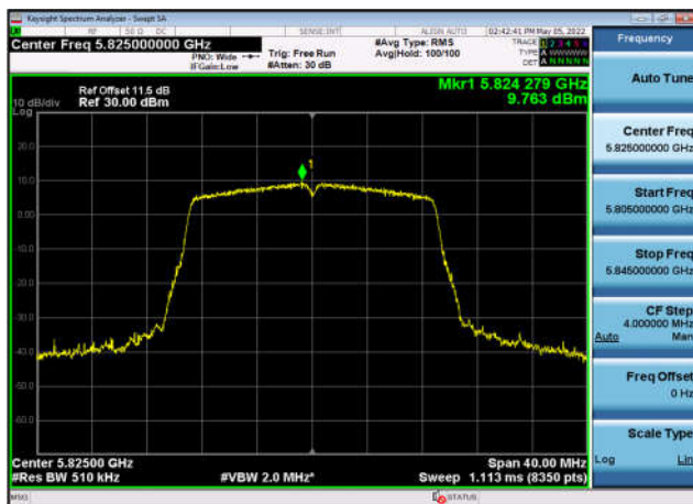
U-NII-3 Power spectral density-802.11 ax(20MHz),5825MHz,Ant2
