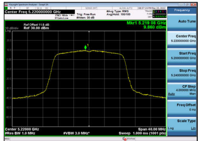
U-NII-1 Power spectral density-802.11 ac(40MHz),5190MHz,Ant0
