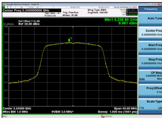
U-NII-1 Power spectral density-802.11 ac(20MHz),5240MHz,Ant0
