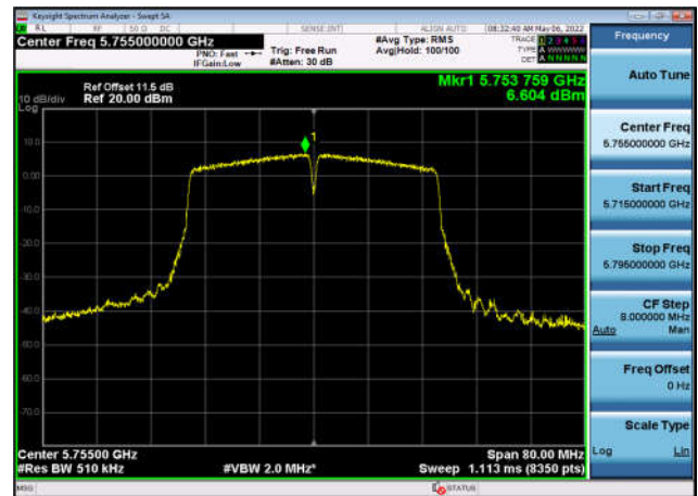
U-NII-3 Power spectral density-802.11 ac(80MHz),5775MHz,Ant1
