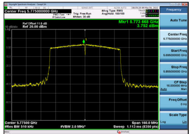
U-NII-3 Power spectral density-802.11 ax(20MHz),5785MHz,Ant0
