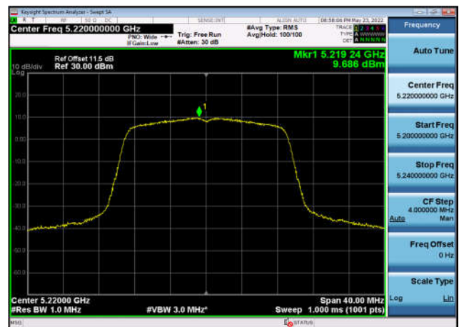
U-NII-1 Power spectral density-802.11 ac(20MHz),5220MHz,Ant1
