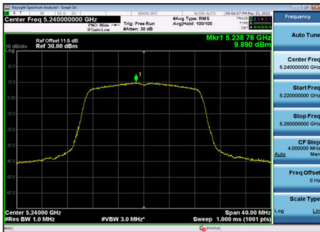
U-NII-1 Power spectral density-802.11 ax(40MHz),5230MHz,Ant2
