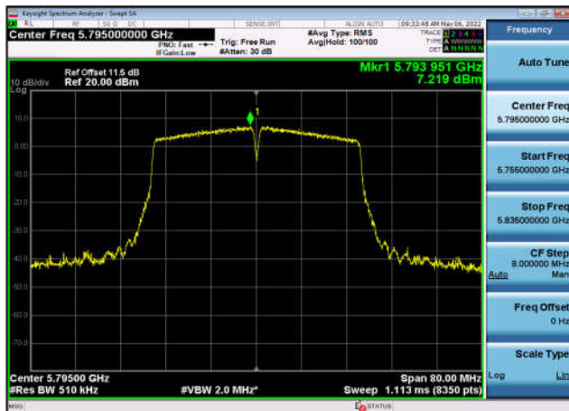
U-NII-3 Power spectral density-802.11 ax(20MHz),5745MHz,Ant3
