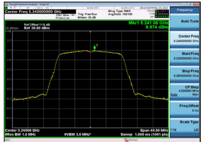
U-NII-1 Power spectral density-802.11 ac(20MHz),5220MHz,Ant0
