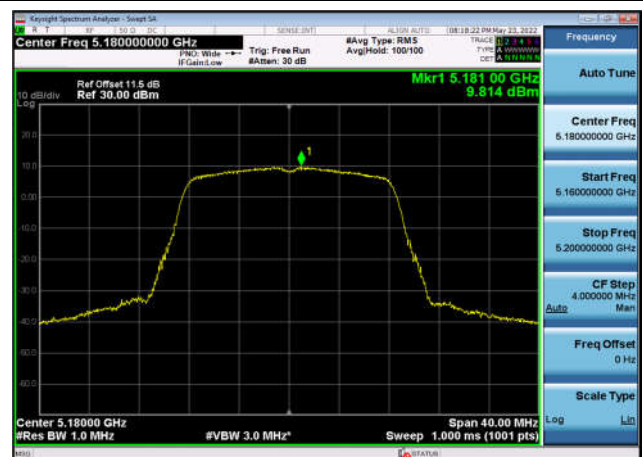
U-NII-1 Power spectral density-802.11 a(20MHz),5180MHz,Ant3
