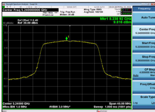
U-NII-1 Power spectral density-802.11 ax(20MHz),5240MHz,Ant0
