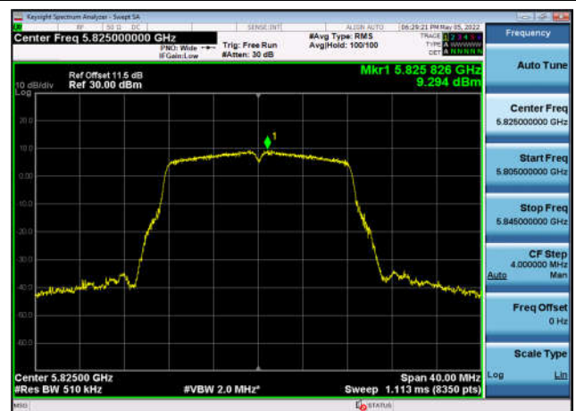
U-NII-3 Power spectral density-802.11 a(20MHz),5825MHz,Ant1
