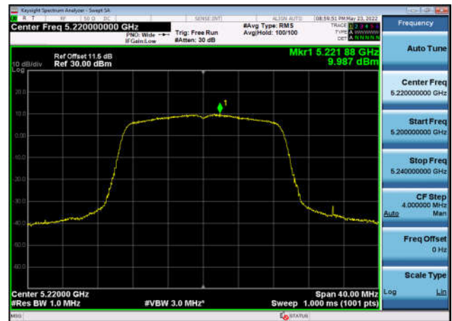
U-NII-1 Power spectral density-802.11 ac(40MHz),5190MHz,Ant3
