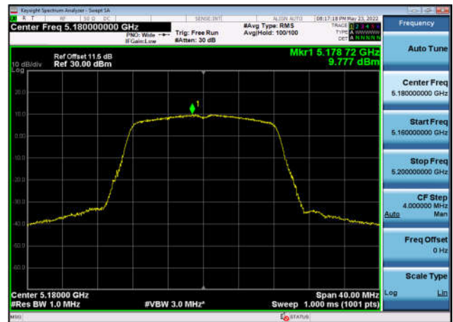
U-NII-1 Power spectral density-802.11 a(20MHz),5240MHz,Ant2
