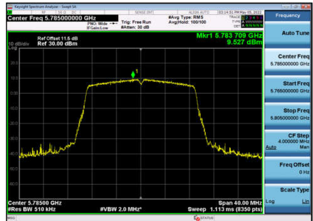
U-NII-3 Power spectral density-802.11 ac(40MHz),5755MHz,Ant1
