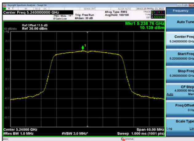
U-NII-1 Power spectral density-802.11 ac(20MHz),5240MHz,Ant3
