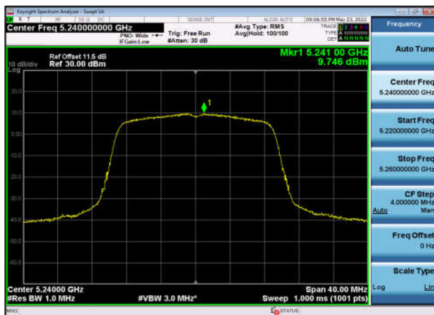
U-NII-1 Power spectral density-802.11 ax(20MHz),5240MHz,Ant3
