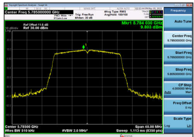
U-NII-3 Power spectral density-802.11 ax(20MHz),5785MHz,Ant3
