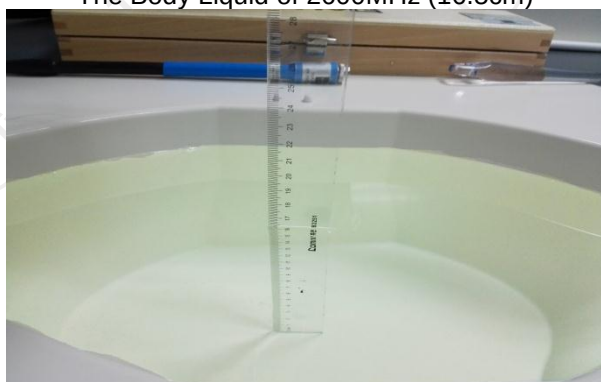
The Body Liquid of 3700MHz (15.2 cm)
