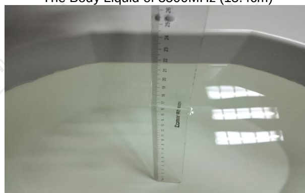
The Body Liquid of 5000-6000MHz (16.5cm)
