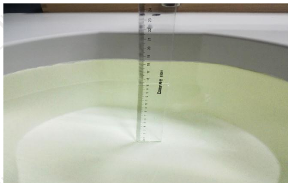
The Body Liquid of 1800MHz (15.2 cm)
