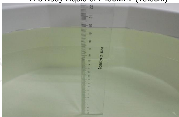
The Body Liquid of 3500MHz (15.4cm)
