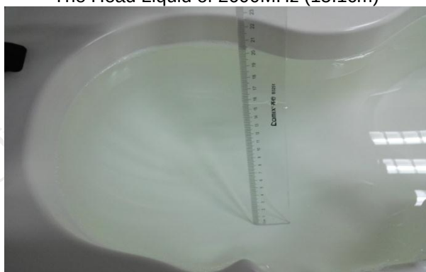
The Head Liquid of 3700MHz (15.6cm)
