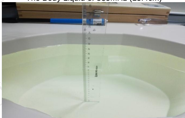
The Body Liquid of 1900MHz (16.4 cm)
