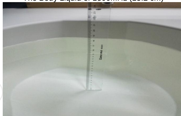
The Body Liquid of 2450MHz (15.3cm)
