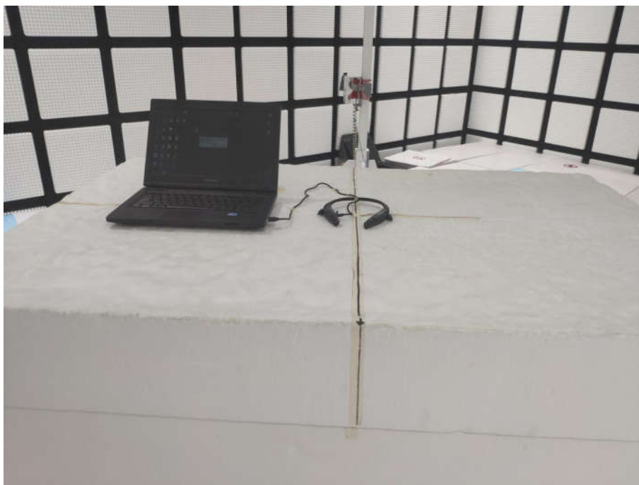
Radiated spurious emission Test Setup-3(Above 1GHz)
