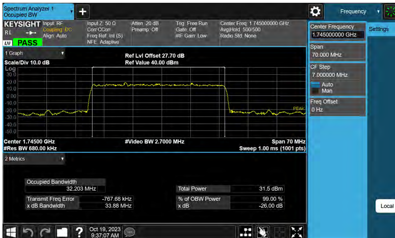
Sub6 n66. Occupied Bandwidth Plot (35 M BW Ch.349000 BPSK Full RB)
