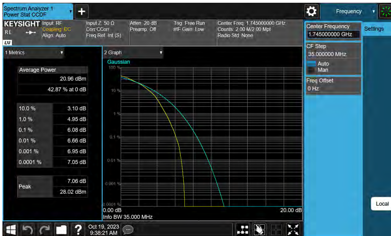
Sub6 n66. PAR Plot (35 M BW_Ch.349000_64QAM_Full RB)
