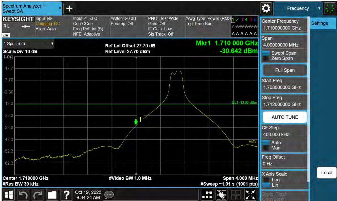
Sub6 n66. Lower Band Edge Plot (35 M BW Ch.345500 BPSK RB 1, Offset 0) -1
