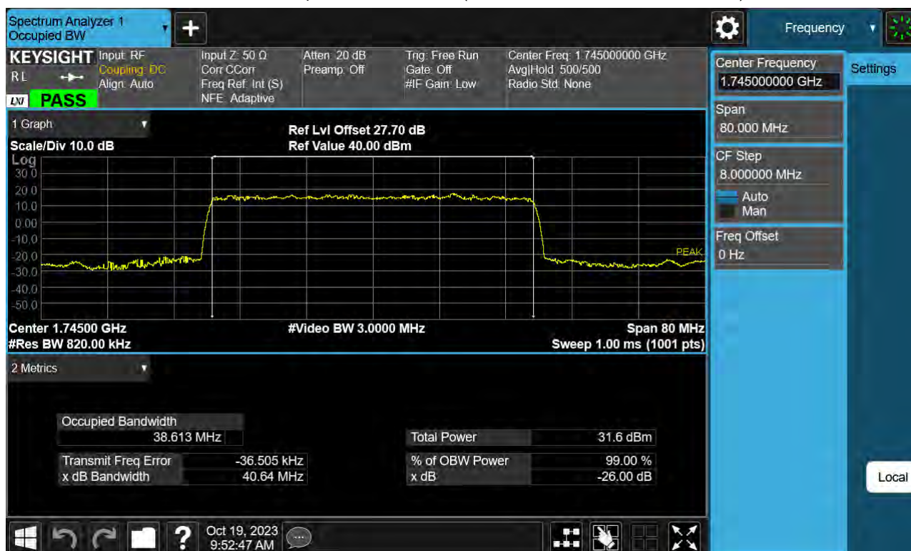
Sub6 n66. Occupied Bandwidth Plot (40 M BW Ch.349000 BPSK Full RB)
