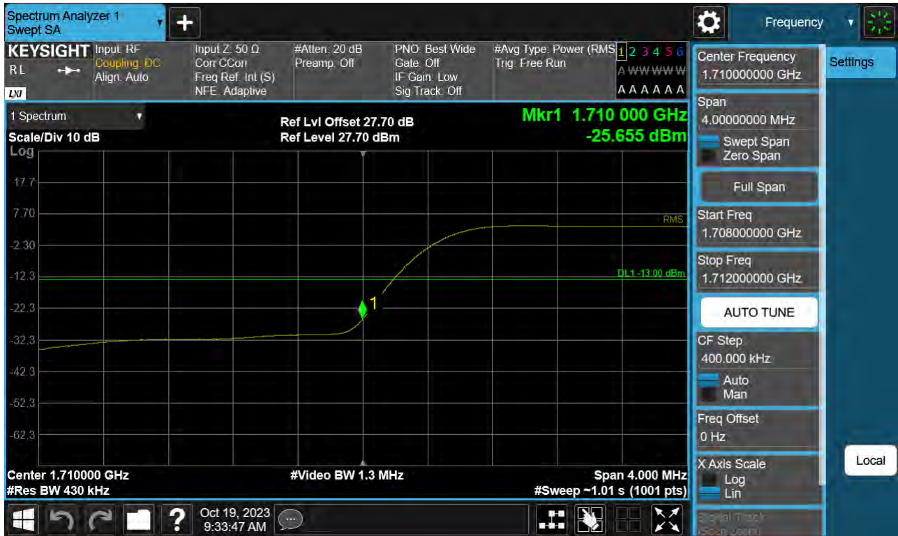
Sub6 n66. Lower Band Edge Plot (35 M BW Ch.345500 BPSK Full RB) -2
