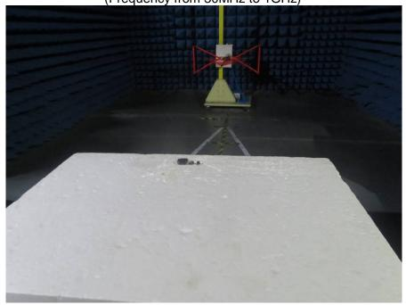
RADIATED EMISSION TEST (Frequency above 1GHz)
