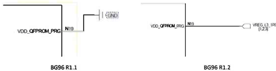
Figure 1: Schematic Designs of BG96 R1.1 and R1.2
