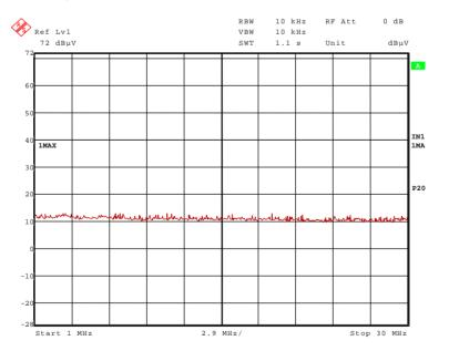
No significant frequencies above the noise floor of the system were found during the preliminary radiated emission test, so no measurements were carried out on the outdoor test site.
