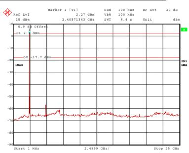
51145173.wmf (conducted emissions 1 MHz to 25 GHz, transmitter at 2441 MHz):
