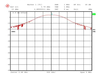
51145164.wmf (maximum peak output power at the upper end of the assigned frequency band):
