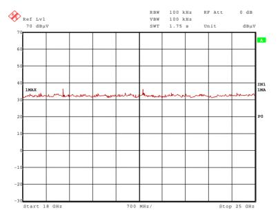
The following frequencies were found inside the restricted bands during the preliminary radiated emission test:
