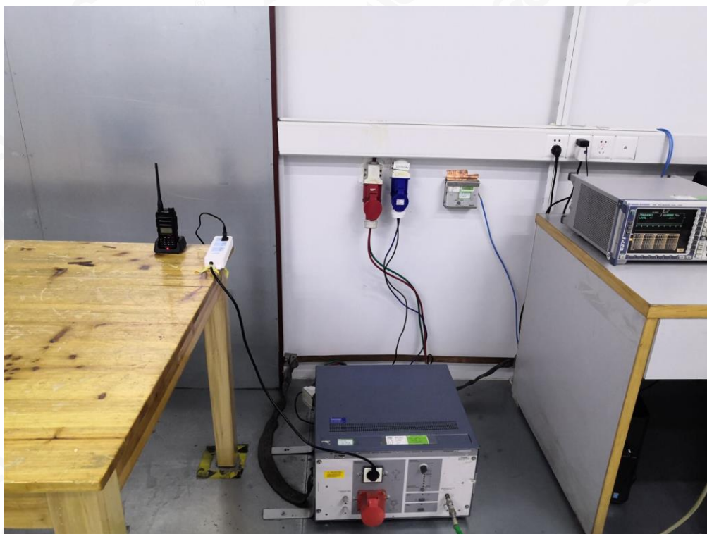
RADIATED EMISSION TEST SETUP-BELOW 1GHZ
