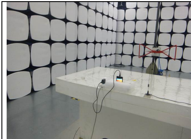
Radiated Spurious Emissions Test Setup Below 1GHz
