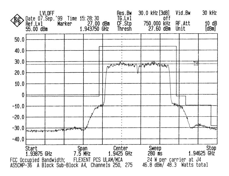
FCC Occupied Bandwidth: Input Chart - PCS B Block, Sub-Block B1, Single Carrier Configuration ULAM/MCA
