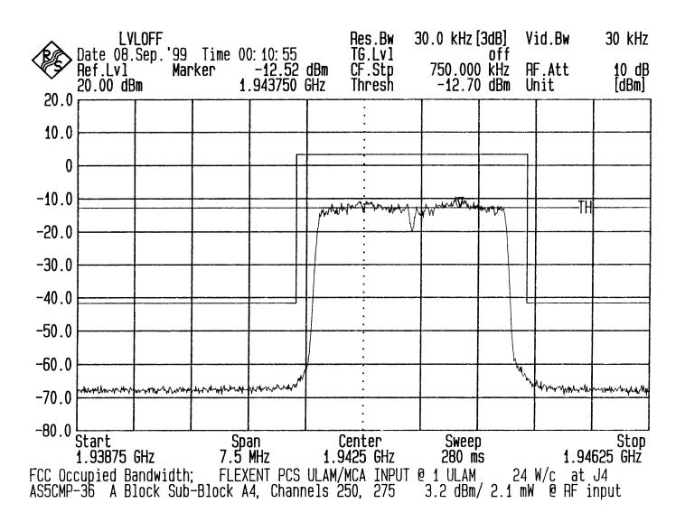
FCC Occupied Bandwidth: Output Chart - PCS A Block, Sub-Block A4, Dual Carrier Configuration ULAM/MCA
