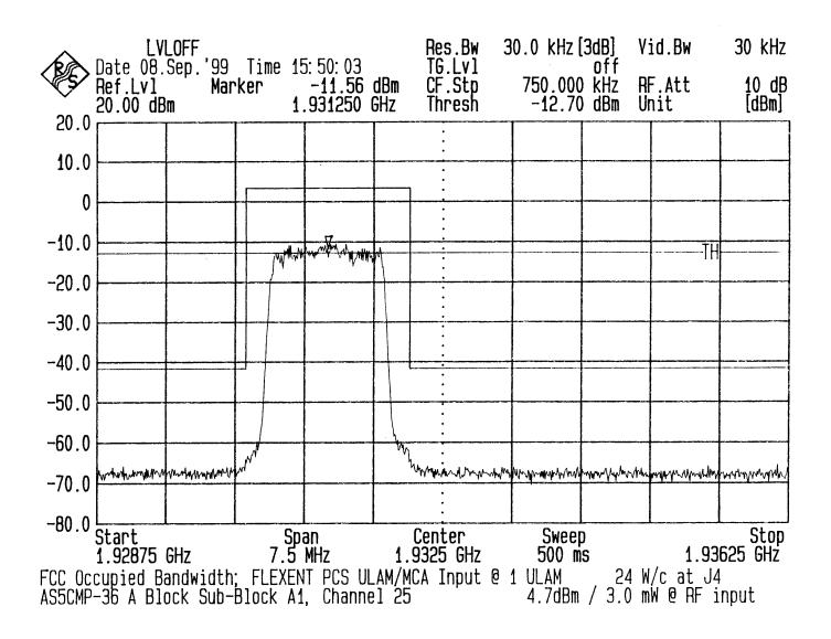
FCC Occupied Bandwidth: Output Chart - PCS A Block, Sub-Block A1, Single Carrier Configuration ULAM/MCA
