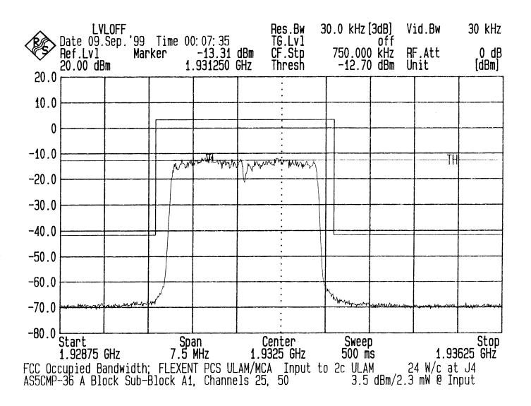
FCC Occupied Bandwidth: Output Chart - PCS A Block, Sub-Block A1, Dual Carrier Configuration ULAM/MCA
