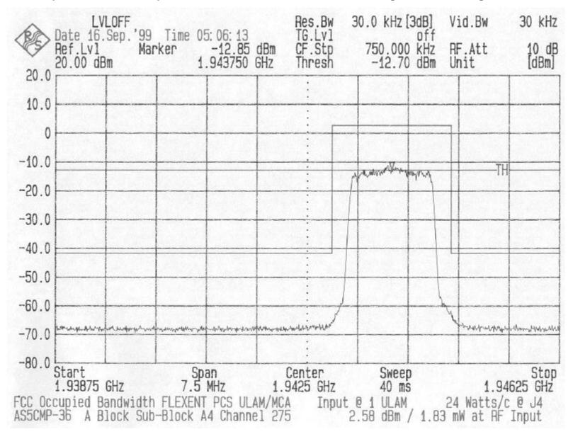
FCC Occupied Bandwidth: Output Chart - PCS A Block, Sub-Block A4, Single Carrier Configuration ULAM/MCA
