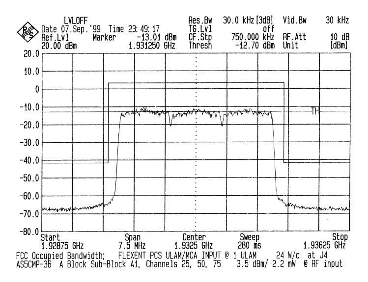
FCC Occupied Bandwidth: Output Chart - PCS A Block, Sub-Block A1, Three Carrier Configuration ULAM/MCA
