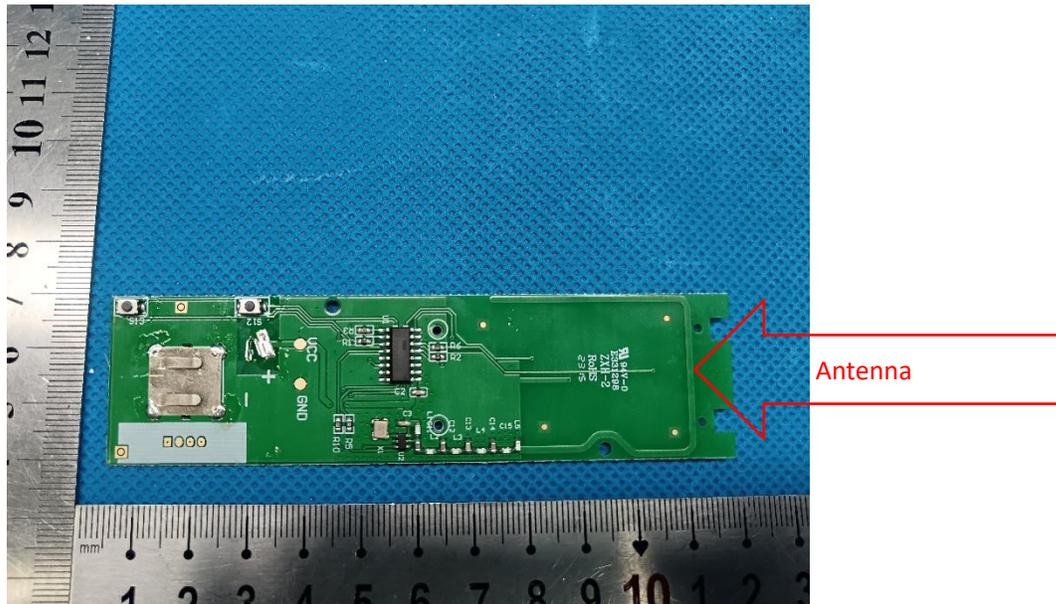
Antenna transmission frequency: 433.92MHz
