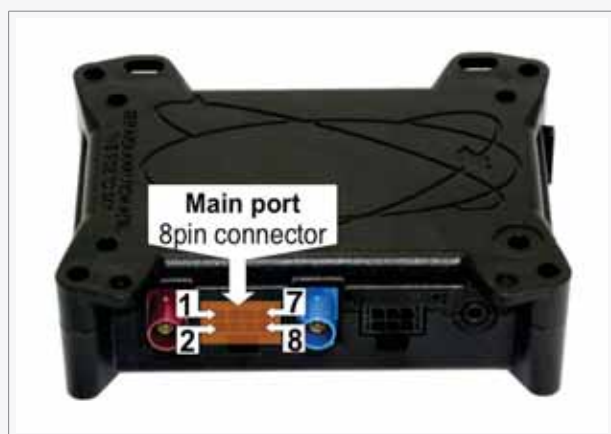
Figure 6: Pin assignments of 8-pin (2x4) connector (Type: MOLEX-43045-08-MICRO FIT)
