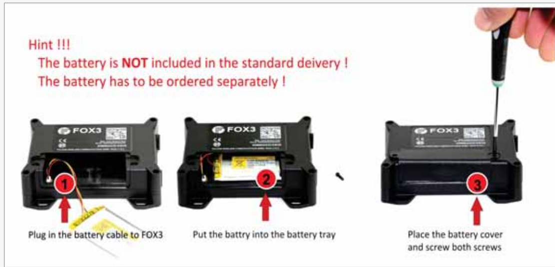
Figure 14.1: Connecting the battery to the FOX3/-3G/-4G devices
