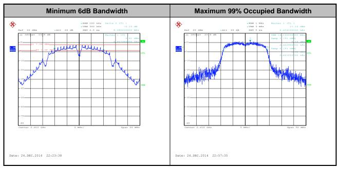
Note: The occupied channel bandwidth is maintained within the band of operation for all of the modulations.
