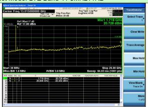
Test Mode: LTE Band 4 / 3MHz /15RB
