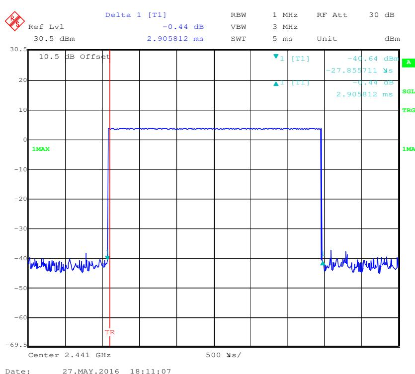
**Pulse time, High Channel, DH5**
