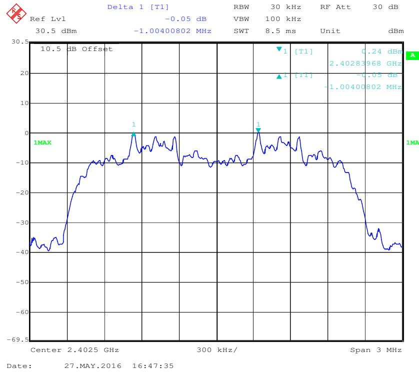
**EDR ( $\pi/4$ -DQPSK): Middle Channel**
