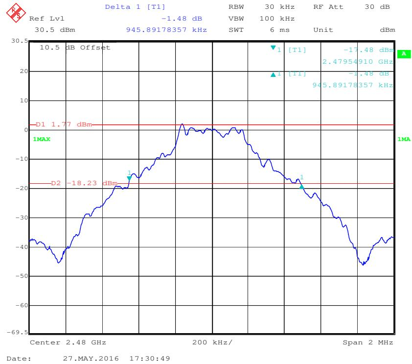
**EDR ( $\pi/4$ -DQPSK): Low Channel**
