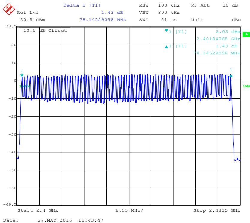
**EDR ( $\pi/4$ -DQPSK): Number of Hopping Channels**
