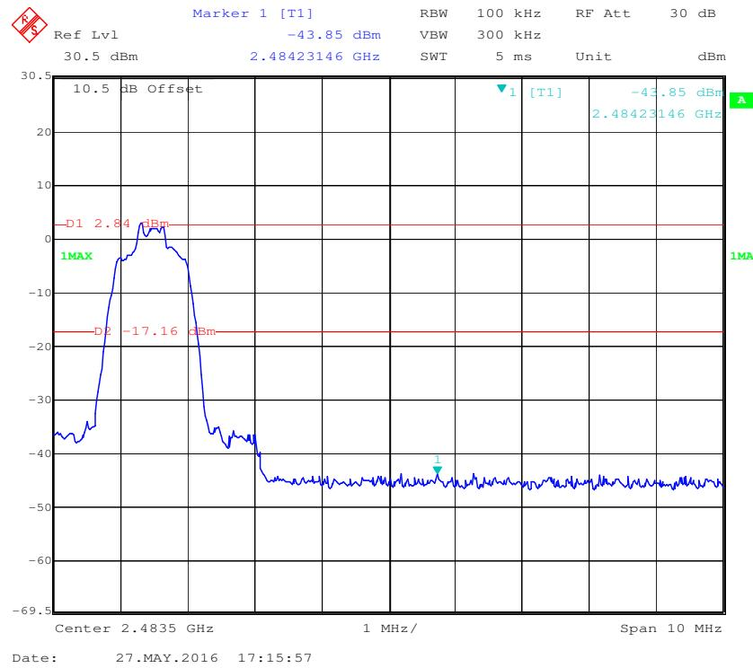
**EDR (8DPSK): Band Edge-Left Side**
