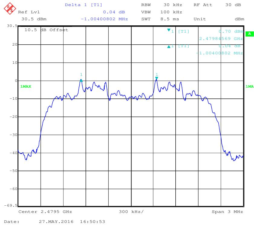
**EDR (8DPSK): Low Channel**
