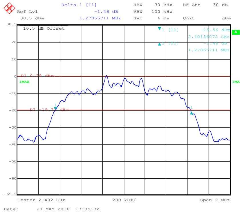
**EDR ( $\pi/4$ -DQPSK): Middle Channel**
