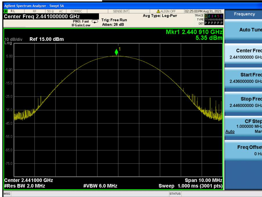
**Peak Output Power****Highest Channel & Modulation : 8DPSK**
