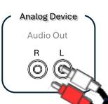
Connect the output of the NERO ARC to a Powered Subwoofer Input or Subwoofer Amp input using an RCA Sub Cable, single or single to dual RCA Sub cable
