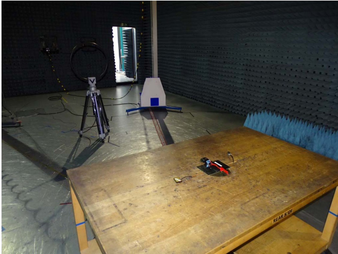
Photo 6: Test setup for radiated measurements (Enclosure, below 30 MHz, intentional radiator §15.209, ANSI C63.10)
