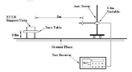
The radiated emission tests were performed in the 3 meters chamber B test site, using the setup accordance with the ANSI C63.4 - 2009. The specification used was the FCC Part 15.209 and FCC Part 15.239.
