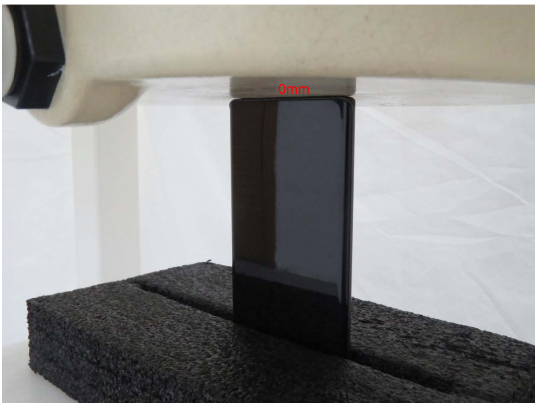
Picture 18: Bottom Edge, the distance from handset to the bottom of the Phantom is 0mm
