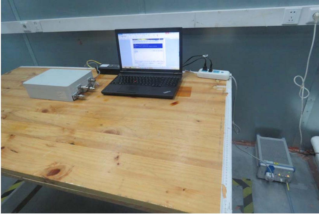
Picture 3 Conducted Emission Test Setup
