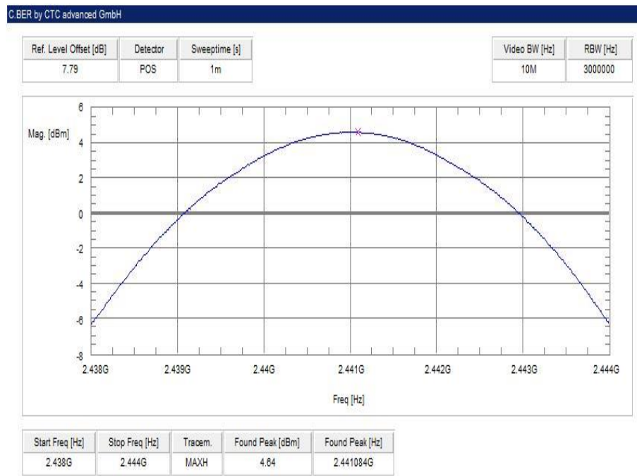
Plot 8: middle channel – 2441 MHz, 8 DPSK modulation
