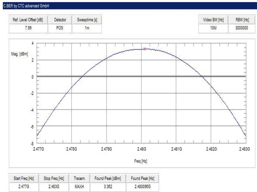
Plot 6: highest channel – 2480 MHz, Pi / DQPSK modulation
