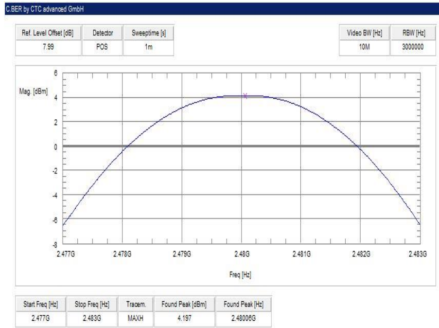
Plot 3: highest channel – 2480 MHz, GFSK modulation
