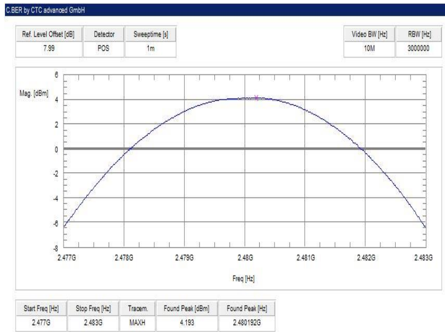
Plot 6: highest channel – 2480 MHz, Pi / DQPSK modulation
