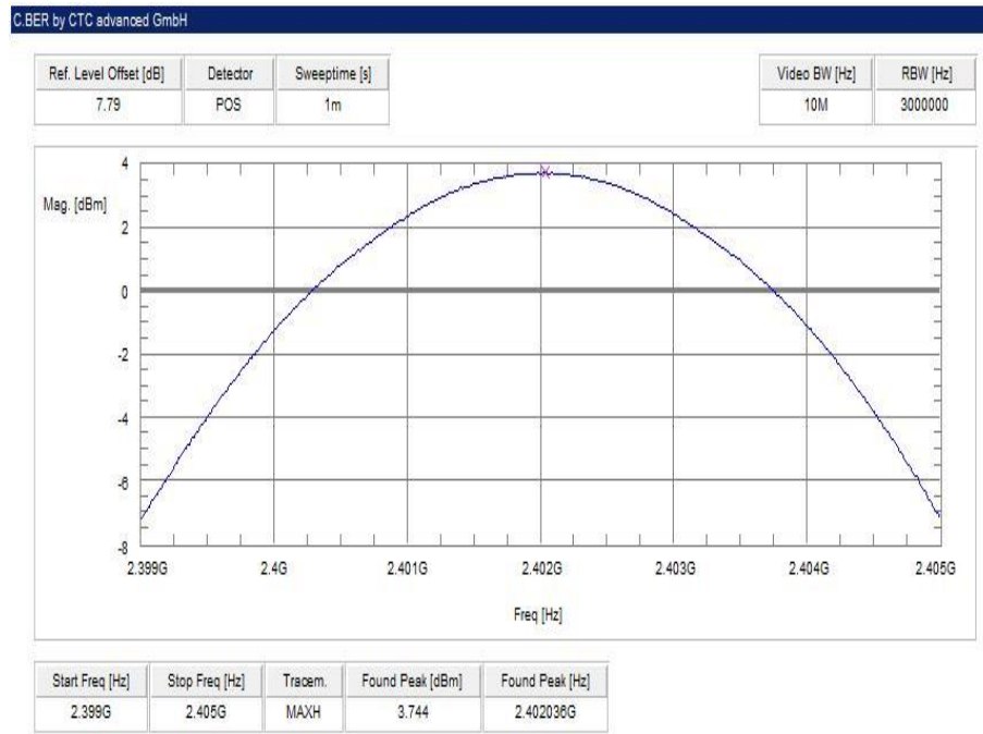
Plot 7: lowest channel – 2402 MHz, 8 DPSK modulation
