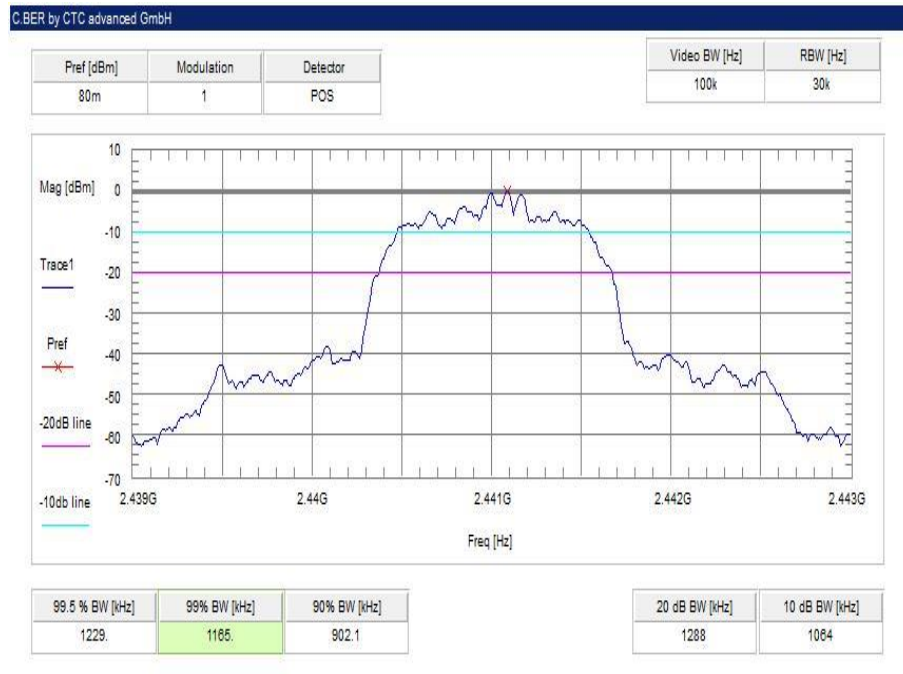
Plot 5: middle channel – 2441 MHz, Pi / DQPSK modulation
