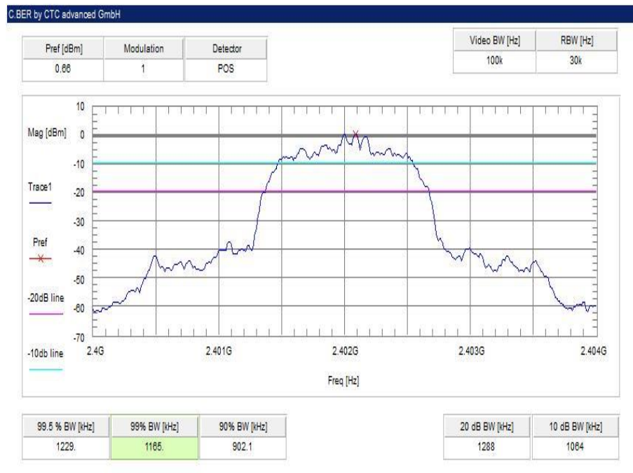
Plot 4: lowest channel – 2402 MHz, Pi / DQPSK modulation
