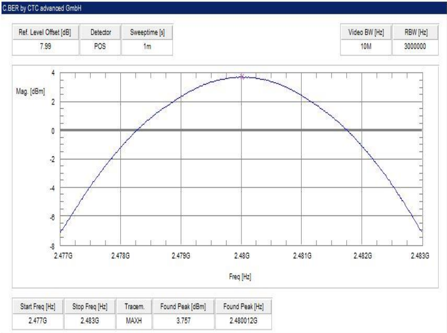
Plot 9: highest channel – 2480 MHz, 8 DPSK modulation
