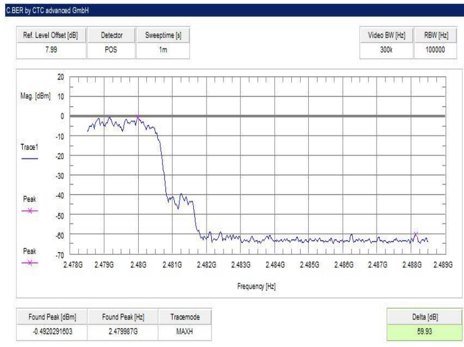
Plot 10: Upper band edge – hopping on, 8DPSK modulation
