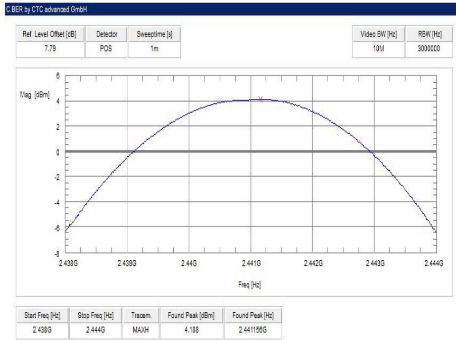
Plot 5: middle channel – 2441 MHz, Pi / DQPSK modulation
