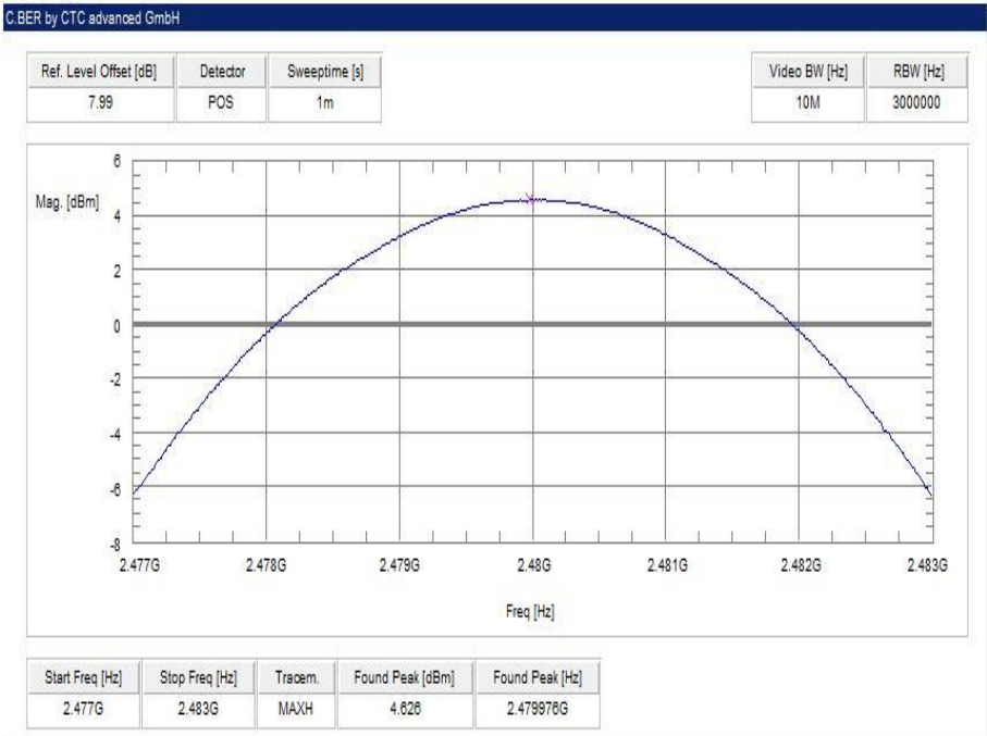
Plot 9: highest channel – 2480 MHz, 8 DPSK modulation
