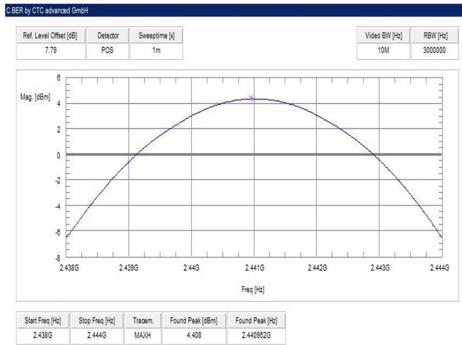
Plot 8: middle channel – 2441 MHz, 8 DPSK modulation
