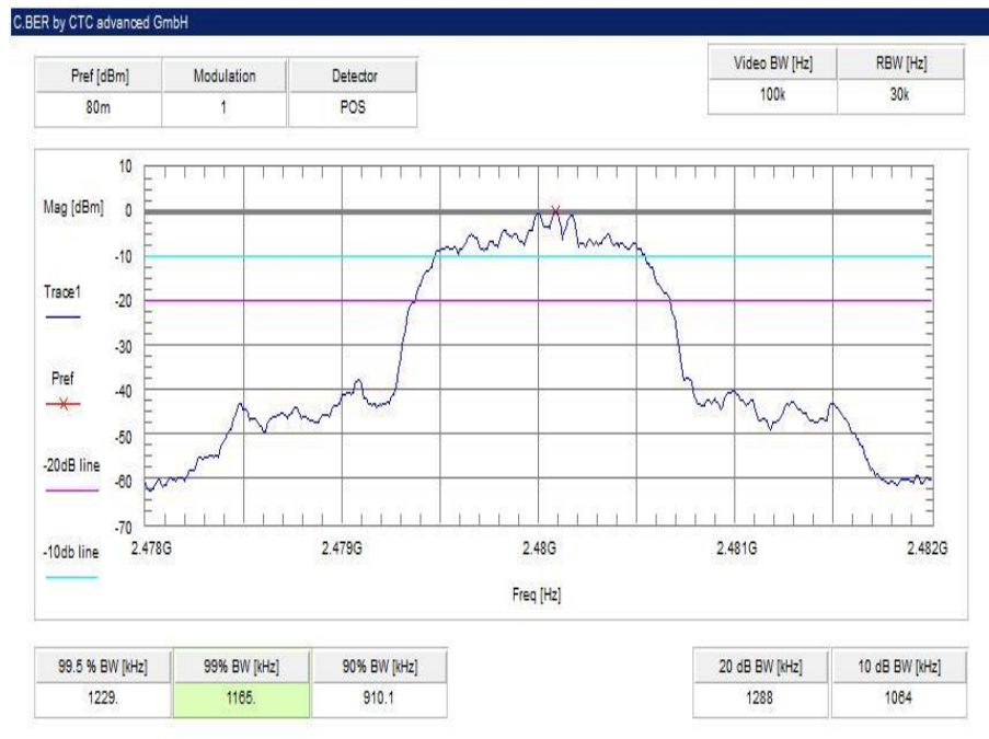
Plot 6: highest channel – 2480 MHz, Pi / DQPSK modulation
