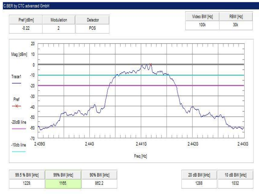
Plot 8: middle channel – 2441 MHz, 8 DPSK modulation
