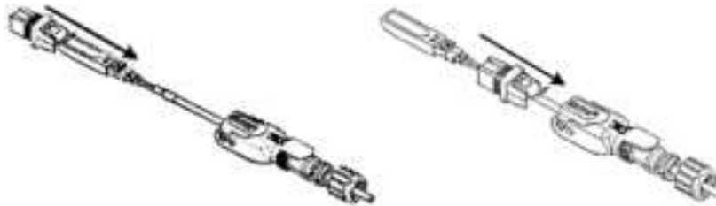
Figure 20: Insert Holder over the Transceiver
