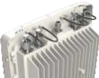
Figure 52: Antenna RF Cables
