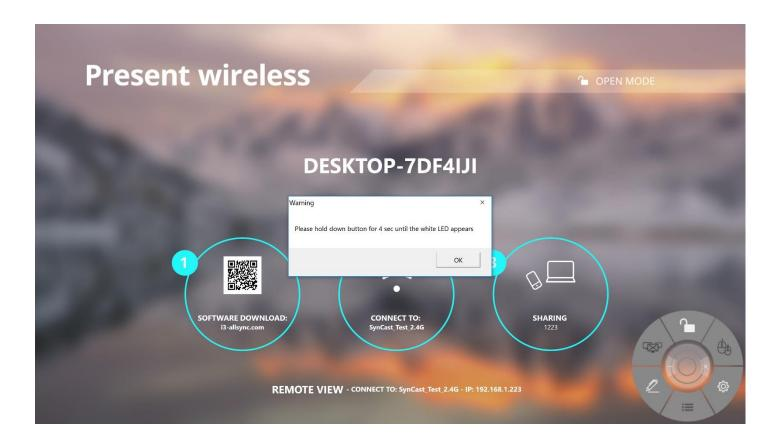
When using the i3ALLSYNC HDMI Tx at the first time, please select "Setting" "WiFi HDMI Tx paring" from Rx device, then hold down the main button of Tx for 4 seconds.
