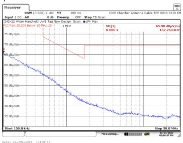
6.4.1.51 Ground Parallel Measurement Antenna – 150 kHz to 30 MHz – Y Axis CH5 16M
