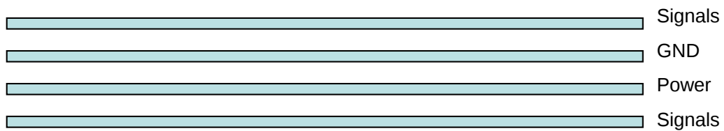
Figure 9: Typical 4-layer PCB construction
