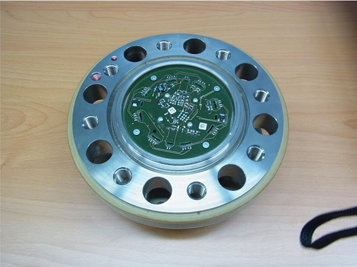
The rotor includes 4 PCB
