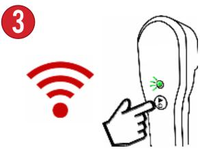
Press the trigger button on the tool, or on the accessory itself to begin reading each tread.
