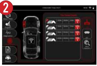
A table will display for each wheel, its measurements, and a trigger button.
