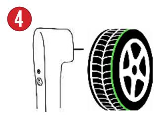
The tool will then prompt you to scan the outer, center, and inner tread. Press the TTD pin into each tread until the tool prompts you to release and move on to the next.
