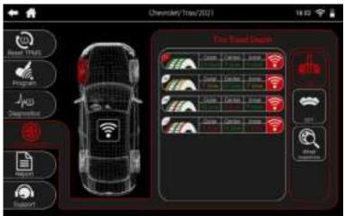
Record and view tire tread readings. Readings are color coded with a tire display to show wear.
