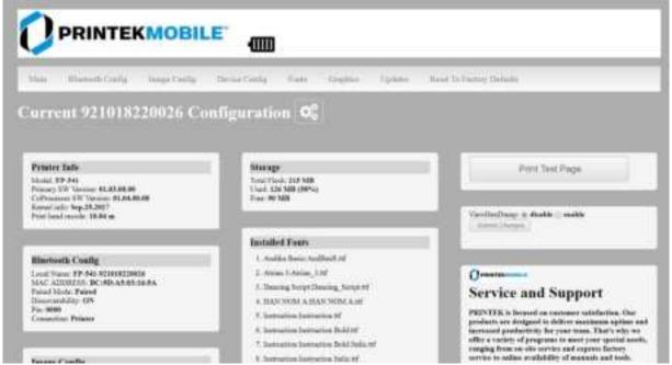
This is an overview of the printer configuration. The battery icon shows the relative charge in the battery. The more bars, the higher the charge. An AC plug will appear in the battery icon when the printer is plugged into an external power source.
