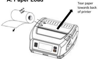
Press Paper door release button to open the paper compartment door. Pull small leader of paper out and close paper door.
