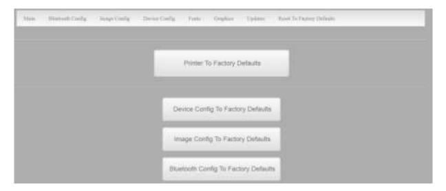
Printer settings can be restored to factory configurations.
