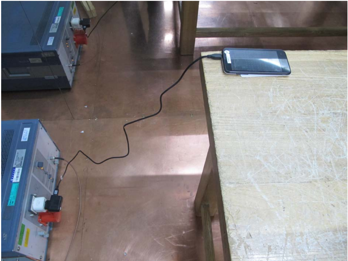
Picture C-3: Conducted Emissions Measurements
