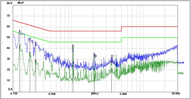
EUT: Smart Projector Phase: L1 M/N.: HY300 Temperature: 26°C
