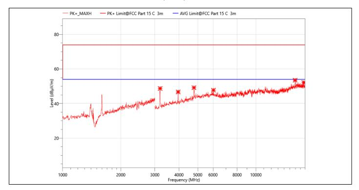
**EUT: Smart Projector Temperature:** 24.3℃ M/N.: HY300 **Humidity:** 54%RH **Power Rating:** Mode: 802.11b 2412MHz AC 120V/60Hz **Test Engineer: Berny Test Time:** 2023-08-30
