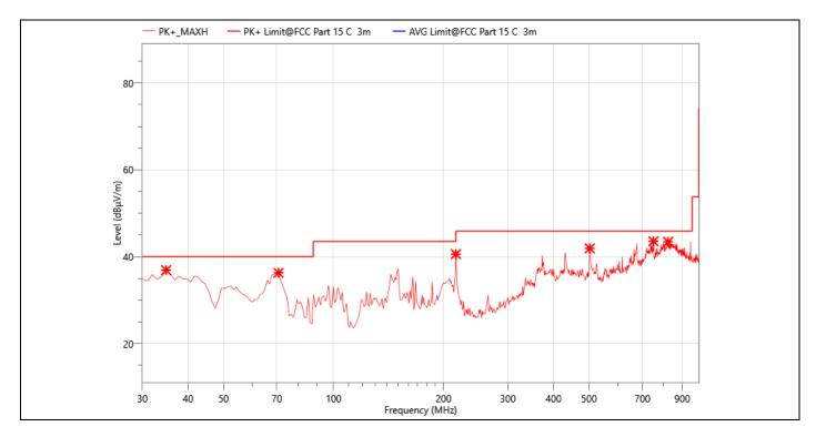
**EUT: Smart Projector Temperature:** 24.3℃ **Humidity:** 54%RH M/N.: HY300 Mode: 802.11b 2412MHz **Power Rating:** AC 120V/60Hz **Test Engineer:** Berny **Test Time:** 2023-08-30
