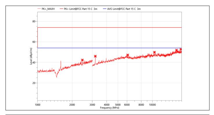
Temperature: **EUT: Smart Projector 24.3℃** M/N.: HY300 **Humidity:** 54%RH **Power Rating:** Mode: 802.11b 2437MHz AC 120V/60Hz **Test Engineer: Test Time:** 2023-08-30 **Berny**
