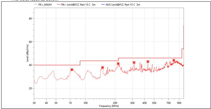
EUT: **Smart Projector Temperature:** 24.3℃ M/N.: **Humidity:** HY300 54%RH Mode: 802.11b 2412MHz **Power Rating:** AC 120V/60Hz **Test Engineer: Test Time: Berny** 2023-08-30
