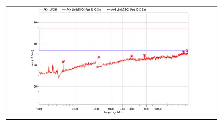
**EUT: Smart Projector** Temperature: **24.3℃** M/N.: HY300 **Humidity:** 54%RH **Power Rating:** Mode: 802.11b 2412MHz AC 120V/60Hz **Test Engineer: Test Time:** 2023-08-30 **Berny**
