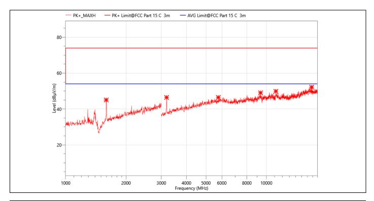
**EUT: Smart Projector Temperature: 24.3℃** M/N.: HY300 **Humidity:** 54%RH **Power Rating:** Mode: 802.11b 2437MHz AC 120V/60Hz **Test Engineer: Test Time:** 2023-08-30 **Berny**
