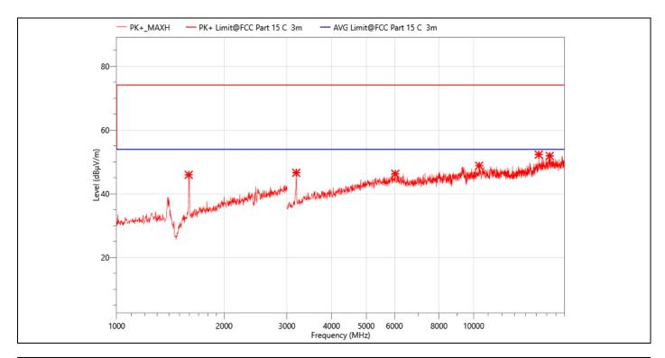
**EUT: Smart Projector Temperature: 24.3℃** M/N.: HY300 **Humidity:** 54%RH **Power Rating:** Mode: 802.11b 2462MHz AC 120V/60Hz **Test Engineer: Test Time:** 2023-08-30 **Berny**
