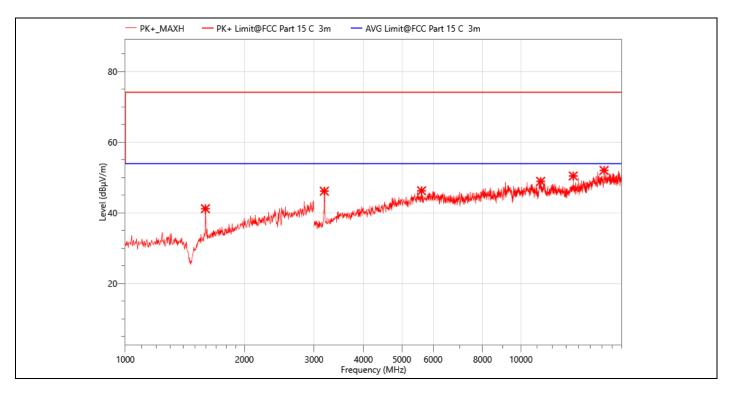
**EUT: Smart Projector Temperature:** 24.3℃ M/N.: HY300 **Humidity:** 54%RH Mode: 802.11b 2462MHz **Power Rating:** AC 120V/60Hz **Test Time:** 2023-08-30 **Test Engineer: Berny**
