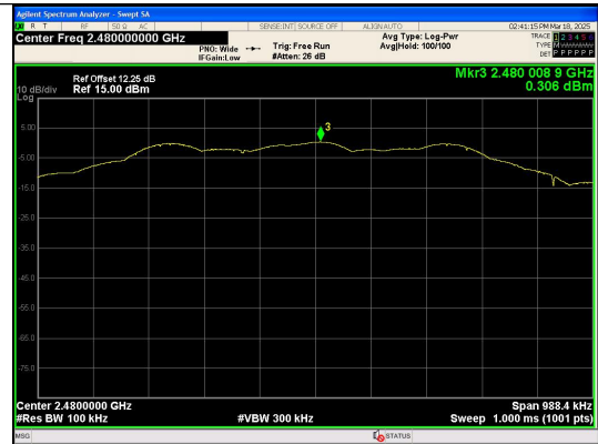
In-Band Reference Level BLE 1M_Channel 39
