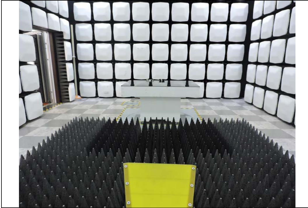
Radiated Emission Test Setup (ABOVE 1 GHz)
