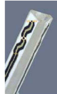
Figure 3.3 Probe Thick-Film Technique
